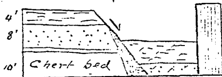
Figure 114. Section of Deschambault limestone exposed at Marble's dam, on Chicot river, St. Outteart. Looking S.W. across stream. See page 22. scale vertical, / 20 feet /
