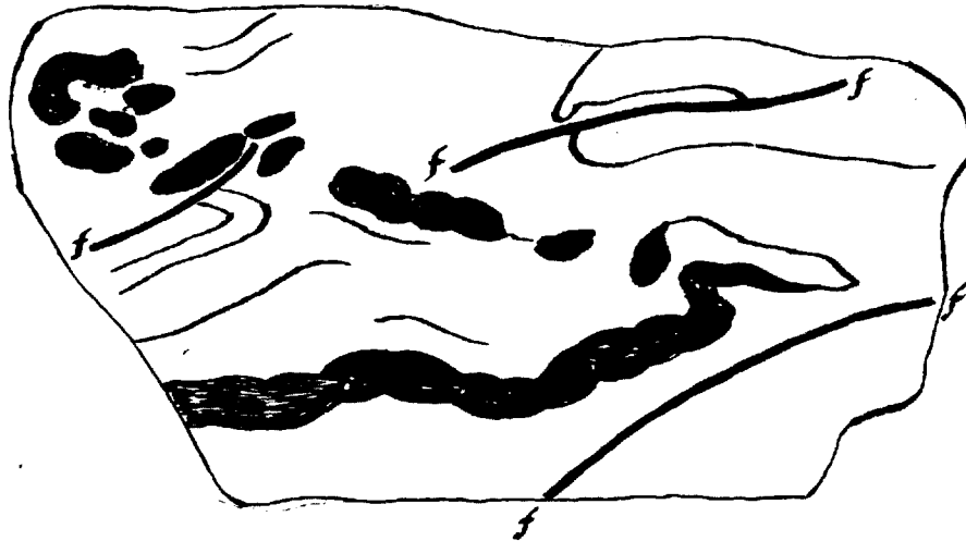
Fig. 8: Highly deformed limestone bed in slates, Rioux quarry, Cowansville. Height of exposure 6 feet. Faults (f-f)
