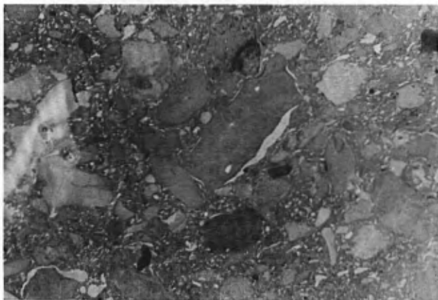
A - Section polie de la brèche argileuse. Polished section of the shale breccia.
