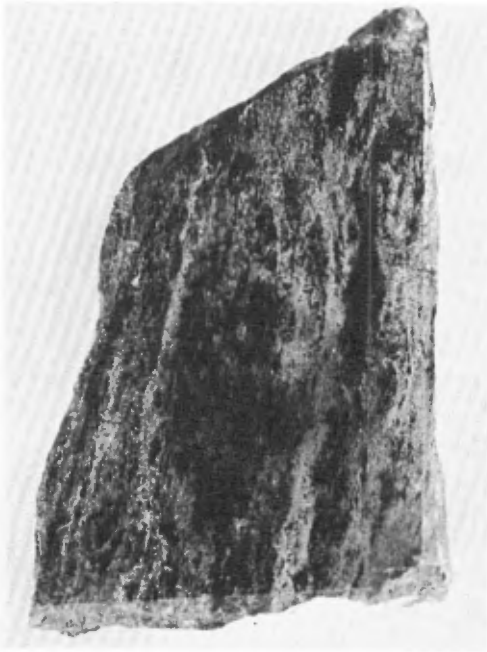
c) Foliate magnetite-pyrite-pyrrhotite. Chlorite folia (black) are intercalated with the sulfides. Compare with sector "B" plate IVa. (Mattagami Lake Mines, x1).
