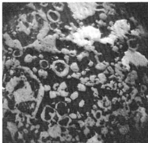
a) Magnetite interstitial to quartz grains and replaced by chalcopyrite, Radiore (x 100).
