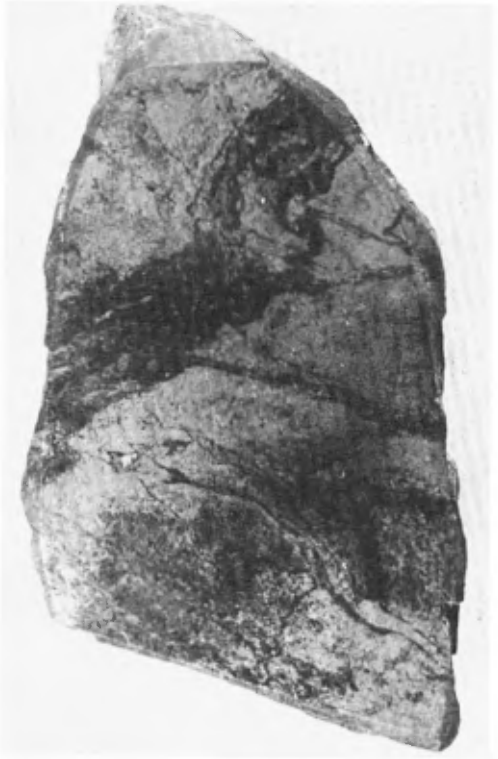
d) Brecciated pyrite with veinlets of magnetite (black). (Mattagami Lake Mines, x1).
