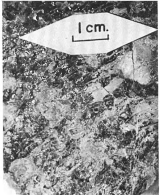
B- Black glass with buff, devitrified areas, this is also a welded tuff and relict flow banding can be seen (top to bottom left in photo). Location: Harrison brook, Raudin twp., Gaspé-South county.
