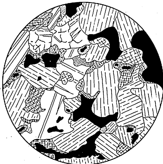
B - Rims of hornblende (stippled) around ore (black) and pyroxene (dashed) in an ilmenite-magnetite gabbro. X 27
