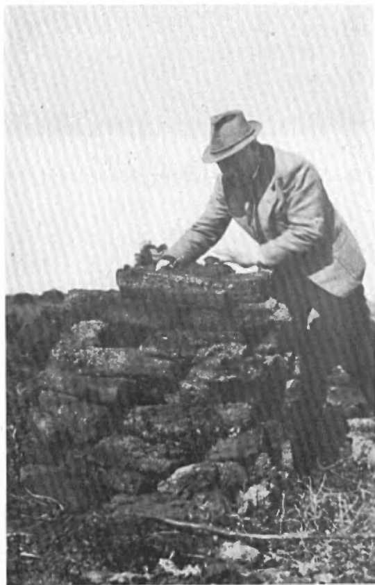
Plate IX—Piling peat blocks into conical heaps. Premier Peat Moss, Limited, Isle-Verte bog.
