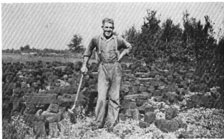
Plate XV—Hand-cutting of peat fuel blocks at St-Isidore.
