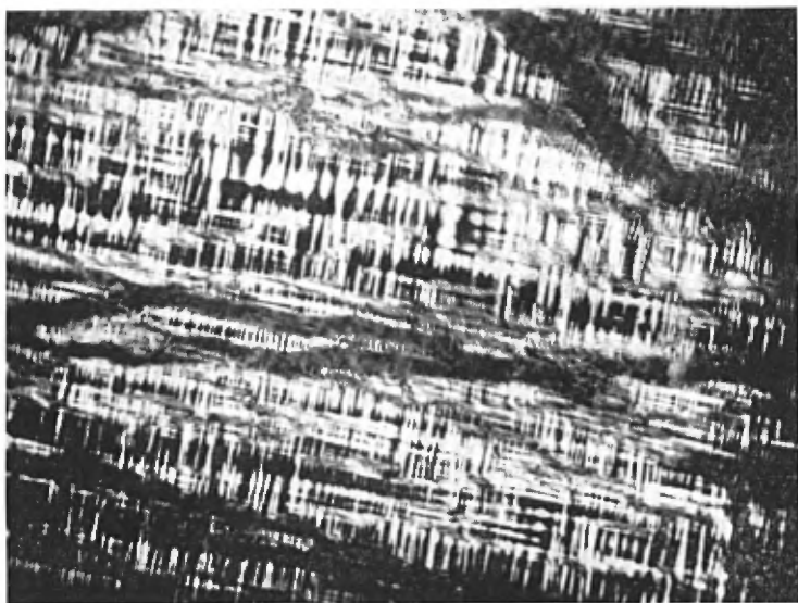
Photomicrograph of thin section of microcline-perthite pegmatite; west point of St. Augustin cove. Crossed nicols, x 51.
