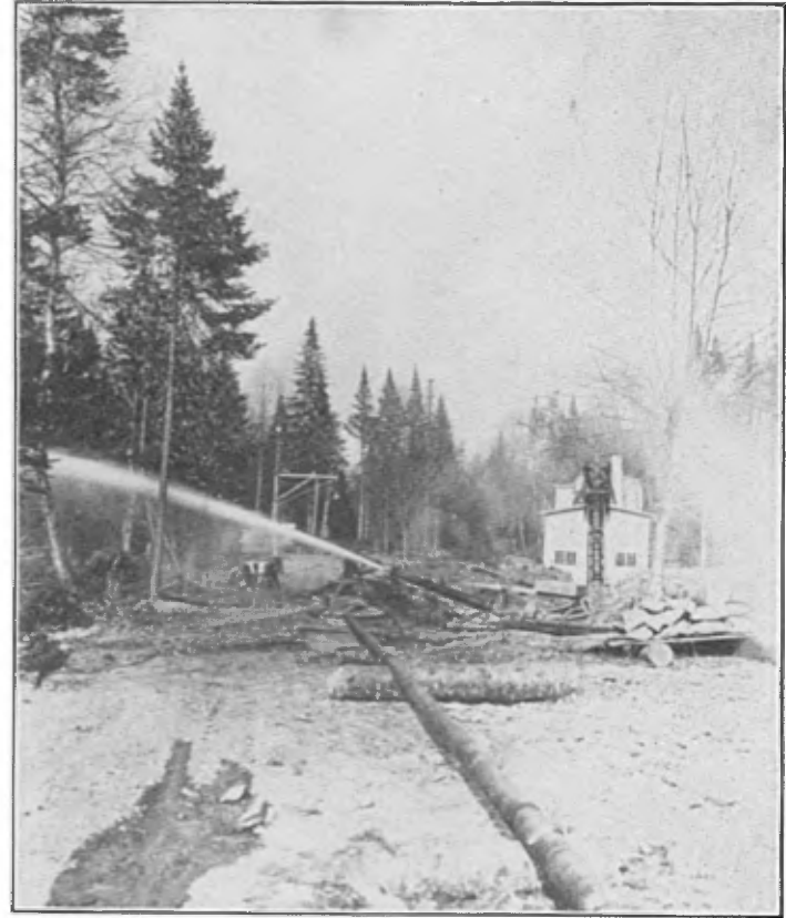
GOLD.—DOMINION GOLD FIELDS, LTD. Monitor, pipe line and elevator on Des Meules creek.
