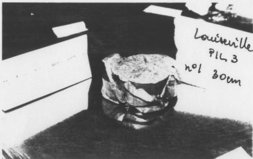
a - Echantillon 5 × 5 cm vertical, W_N = 32,6
