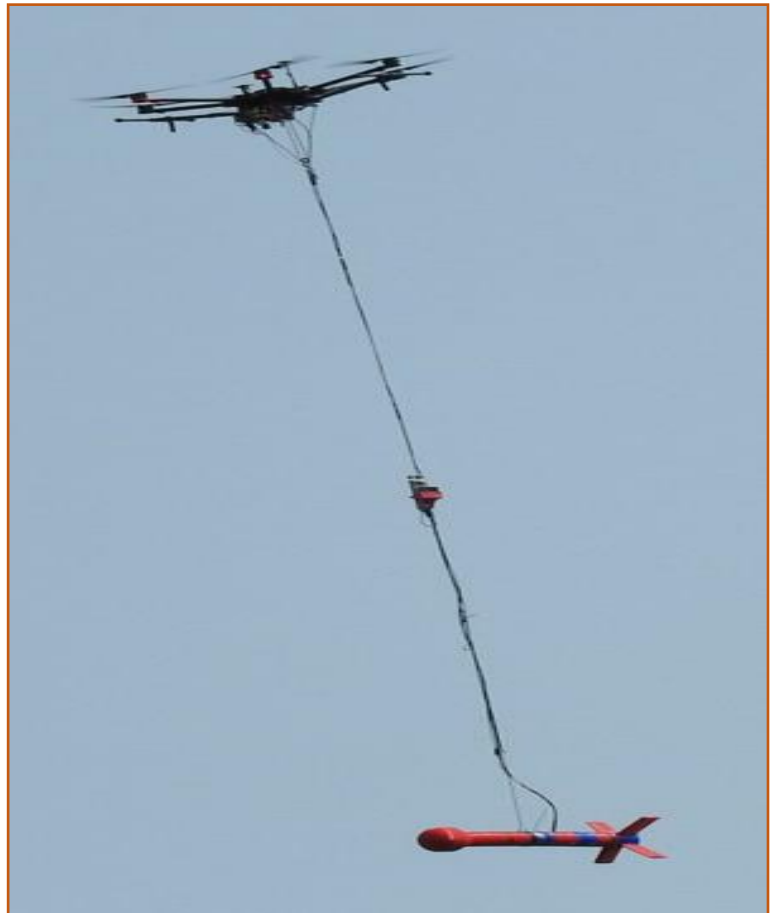
Figure 12. Devbriio UAV-Multicopter with CS-VL magnetometer.
