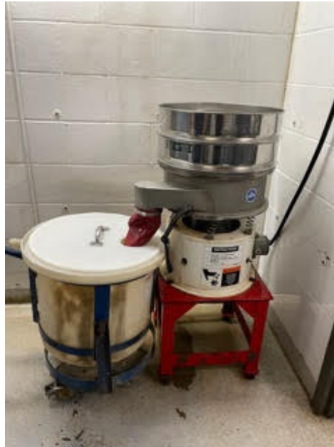
Figure 28: Electric Sweco Vibro-Energy Separator (Model LS18S5P3).
