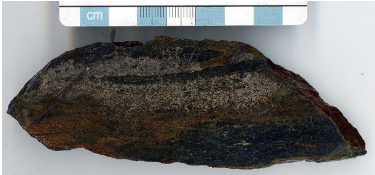
Photo 18: Lac Bruno boulder field – cut hand sample, amphibolite with abundant pyrrhotite
