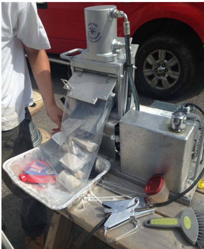
Figure 11. Sample cutted and placed in plastic bag with tag
