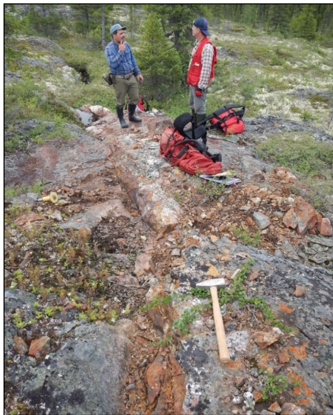
Figure 10. The NW-SE rusty quartz vein known as Esker B2 showing. Sample #E40459 returned 17.86 g/t Au, 100.1 g/t Ag, 0.12% Cu, 10.02% Zn and 27.90% Pb. The host rock corresponds to basalts.
