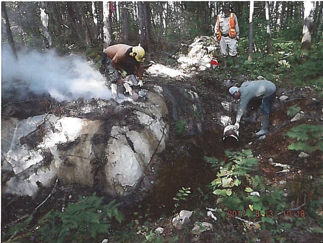
Photograph 9: Saw cutting across mineralized intrusive contact zone at Mason's outcrop northwest of the Copper pit.
