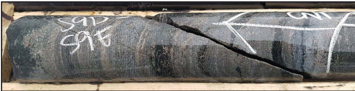
Photograph 4: OSK-TR-17-011, close-up of the 50 cm thick sulphide banded iron formation that returned 1.83 g/t Au over 50 cm.
