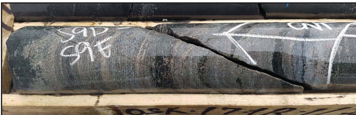
Photograph 2: OSK-TR-17-011 from 86.9-87.4 m, sulphide banded iron formation with 15-20% pyrrhotite as stringers and disseminations.
