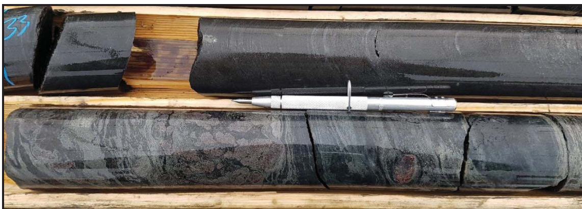
Photograph 6: OSK-TR-17-013, from 34.1-34.8 m, weak biotitization and calc-silicate alteration, moderate chloritization and strong pervasive silicification with 1-2% disseminated pyrrhotite.
