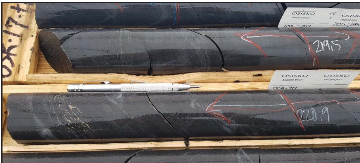
Photograph 5: OSK-TR-17-012, from 219.5-220.9 m, 3 to 5% pyrrhotite as dissemination and stringers with weak pervasive silicification and chloritization.
