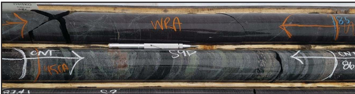
Photograph 1: OSK-TR-17-011 from 86-86.5 m, silicate banded iron formation with traces to 2% of disseminated pyrrhotite.
