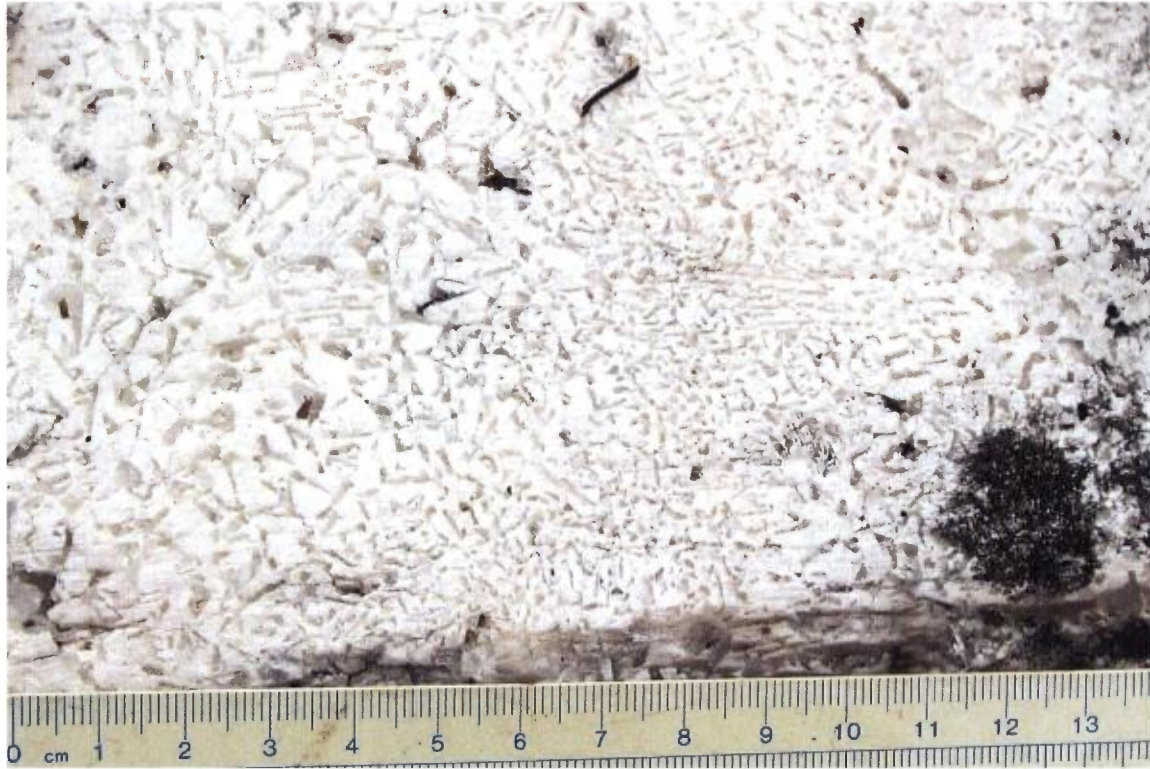
Example of graphic granite (white feldspar and grey quartz) on ridge above Canspar Pit #6
