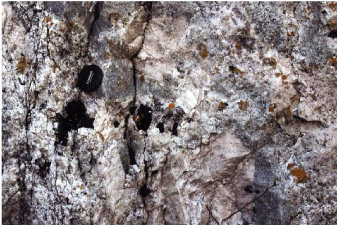
Example of 'fine grained pegmatite', East Mill Cut (Canspar pit #2) - grey sections contain biotite
