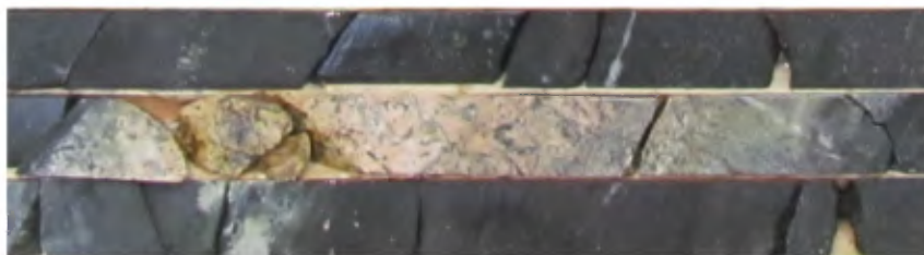
Picture 41: DDH LD-13-04 81.78 m. Granophyre xenolith in layered ferrogabbro.
