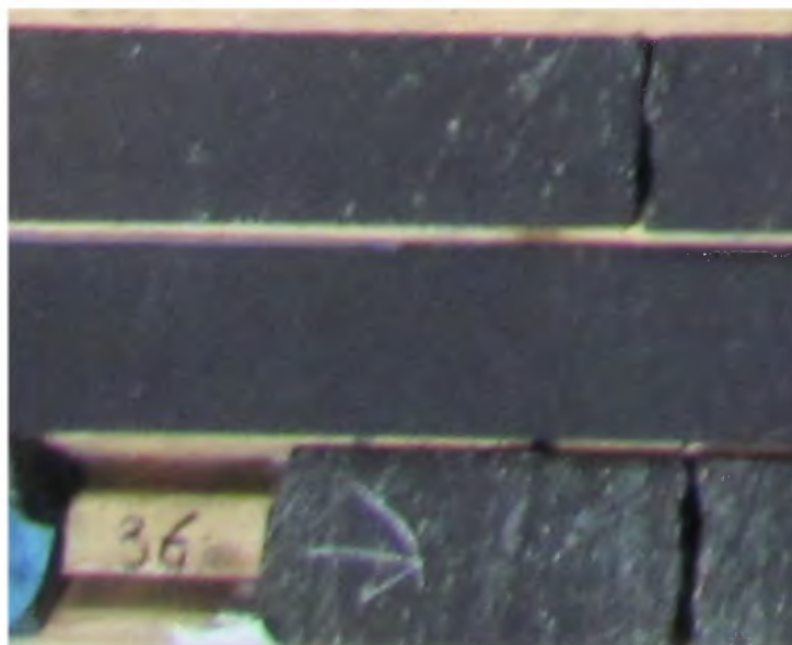
Picture 8: DDH LD-13-01 36.00 m. Mineralized layered zone.
