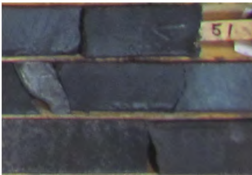
Picture 37: DDH LD-13-04 51.00 m. Mineralized layered zone.
