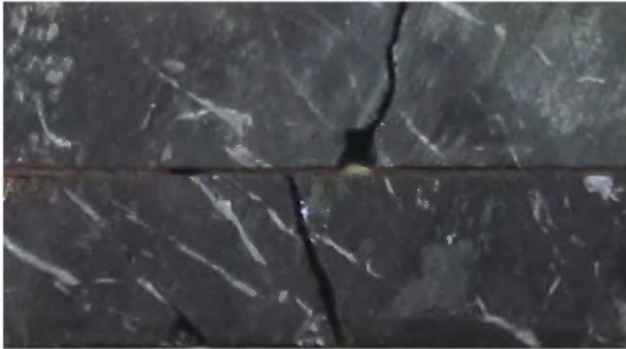
Picture 28: DDH LD-13-03 92.5 m. Carbonate veinlets in ferrogabbro.
