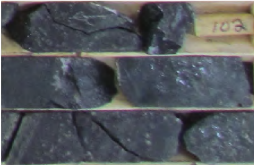
Picture 30: DDH LD-13-03 102.00 m. Mineralized layered zone.
