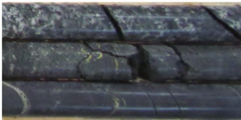
Picture 10: DDH LD-13-01 83.00 m. Dyke of fine grained gabbro in anorthositic gabbro.
