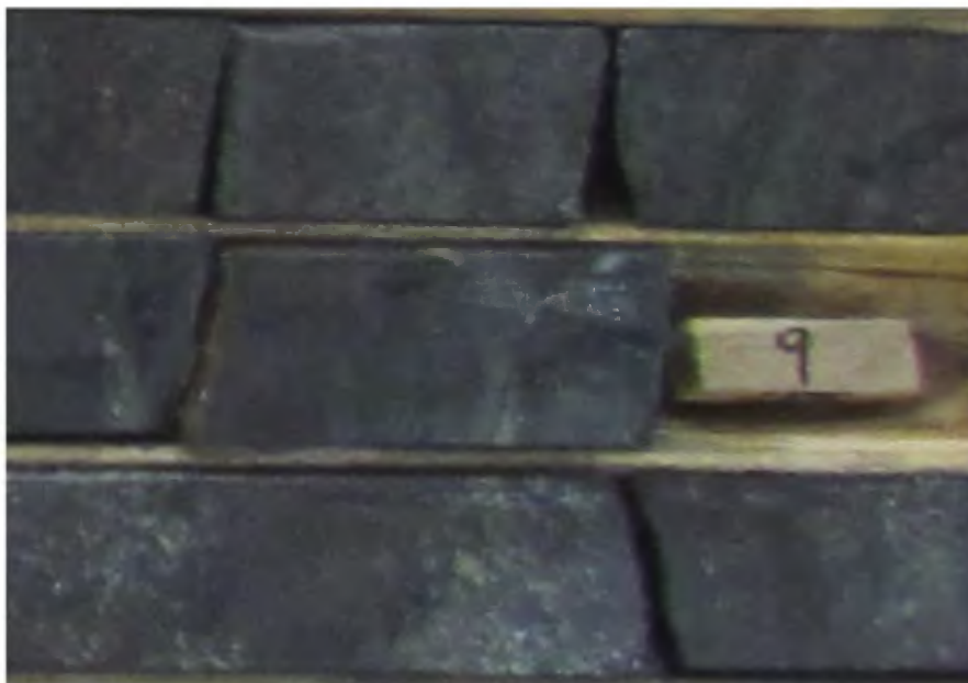
Picture 25: DDH LD-13-03 9.00 m. Mineralized layered zone.
