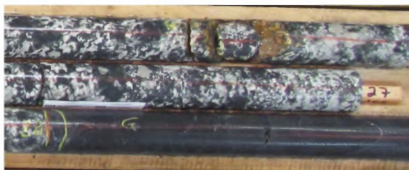
Picture 36: DDH LD -13-04 28.30 m. Contact between a fine grained gabbro dyke and gabbroic anorthosite.
