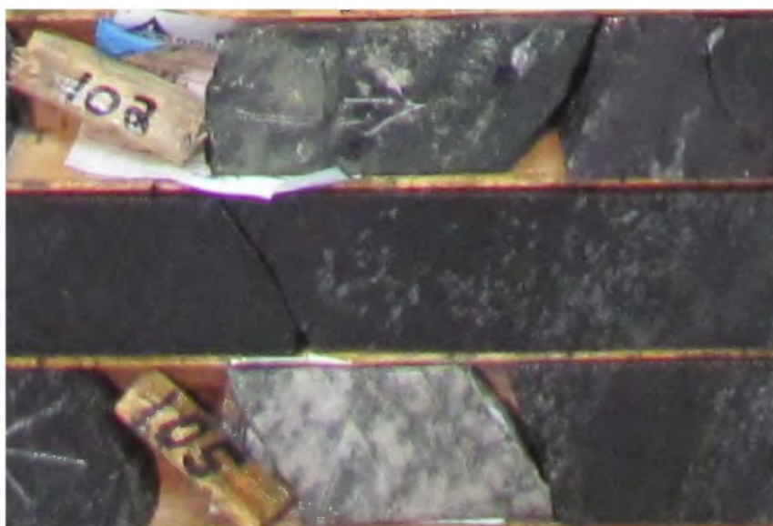
Picture 43: DDH LD-13-04 102.00 m. Mineralized layered zone.
