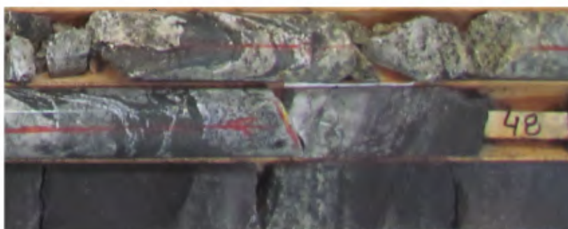
Picture 38: DDH LD-13-04 48.00 m. Injections at the contact between ferrogabbro and anorthosite.
