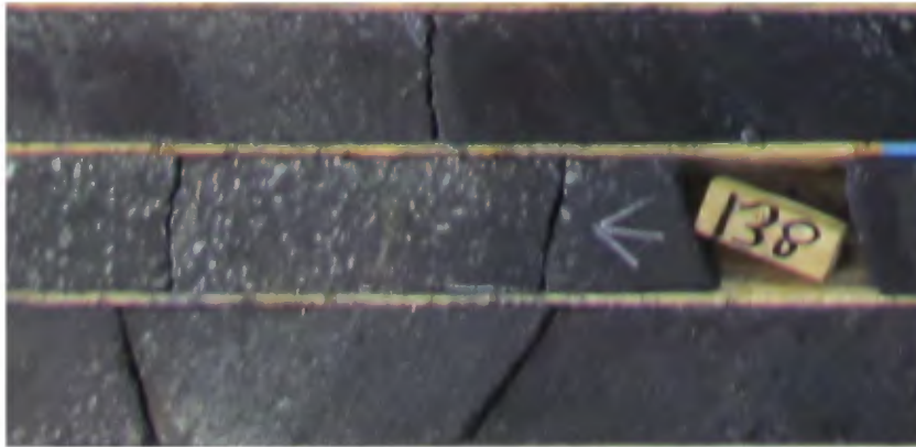
Picture 23: DDH LD-13-02 138.00 m. Magnetite layered with ferrogabbro.
