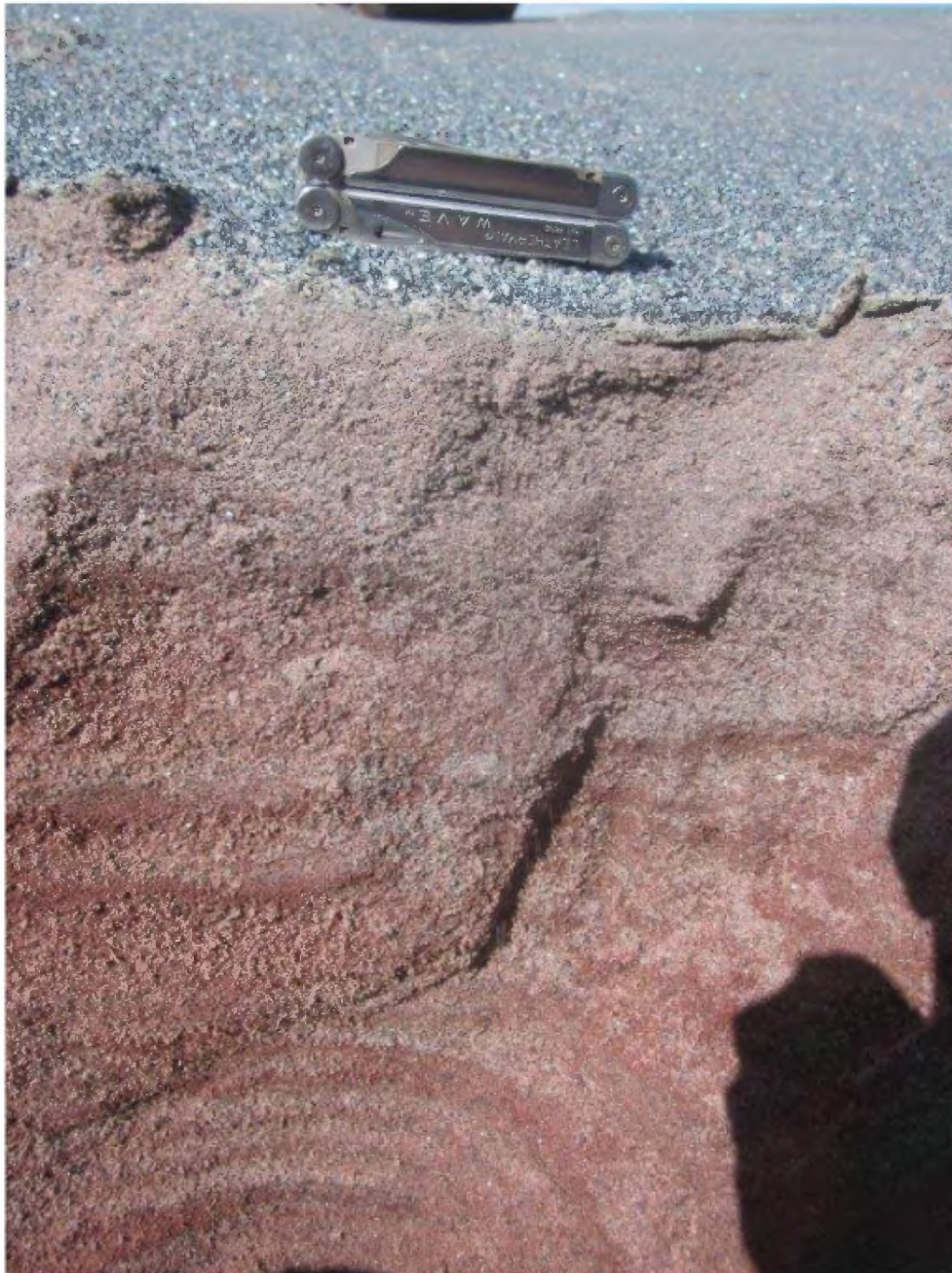
Plate 4: August 2013 sample pit profile - Lac Jeannine Lake tailings. Grey material on surface consists of hematite grains (1-2 mm).
