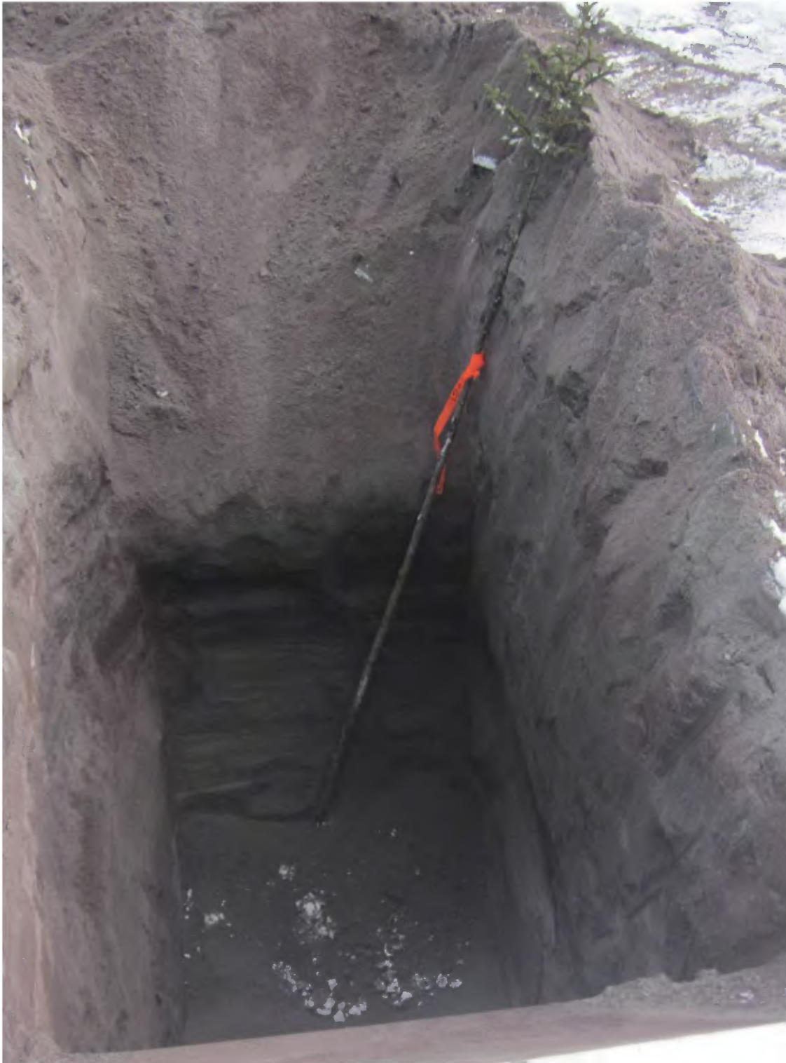
Plate 6: Bulk-sample pit - Lac Jeannine Lake tailings
