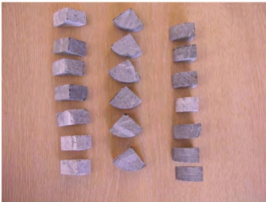
Figure 3 – Orientations of Pieces for Breakage (Cut Core Method)
