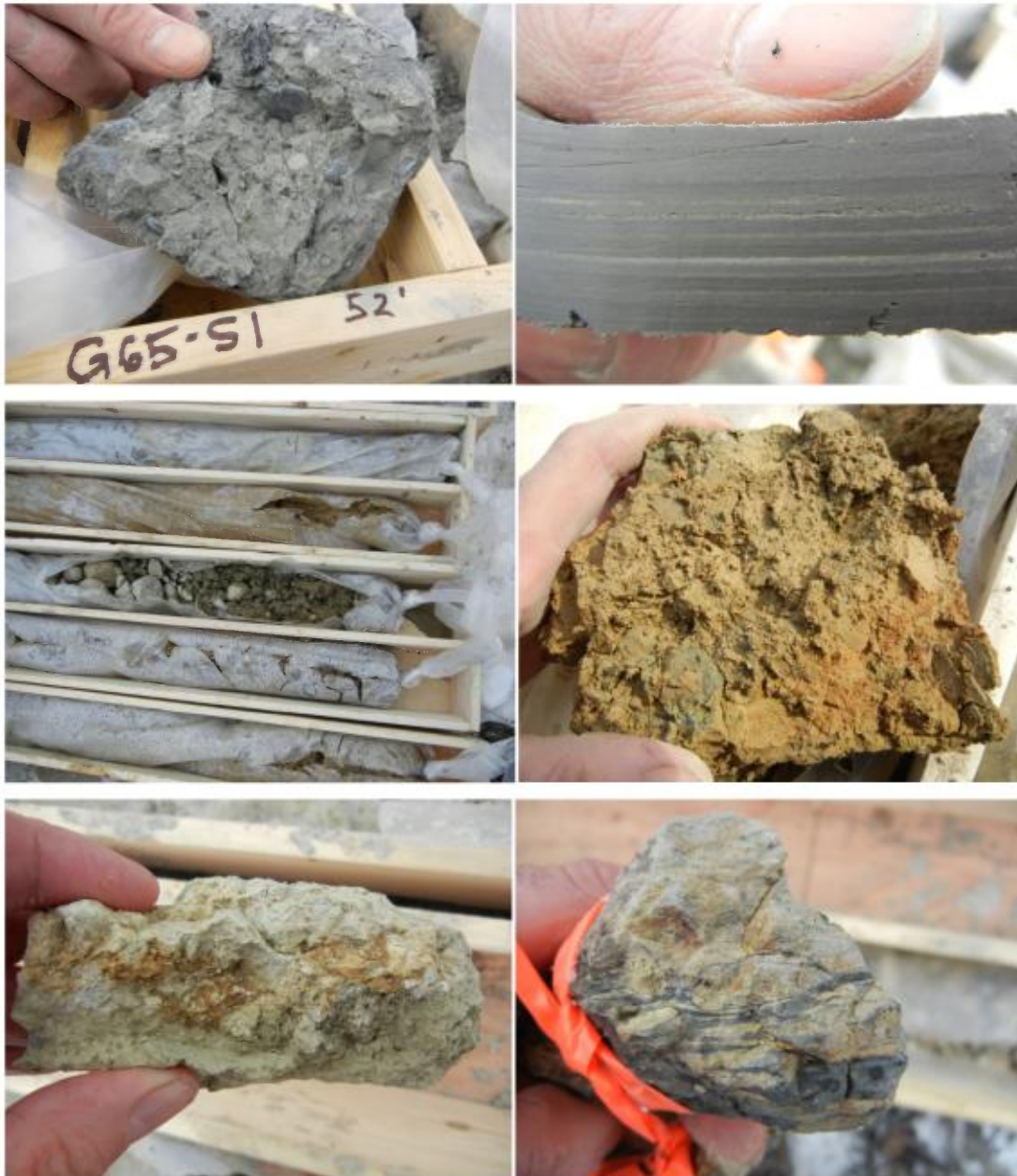
Figure 5. Pictures of sedimentary units. From top left to lower right : Detail of the grey silty diamict (Unit 1), finely laminated silt and fine sand (unit 2), cores and detail of the brown clayey diamict (unit 3), brownish beige alterite (unit 4) and its underlying bedrock.
