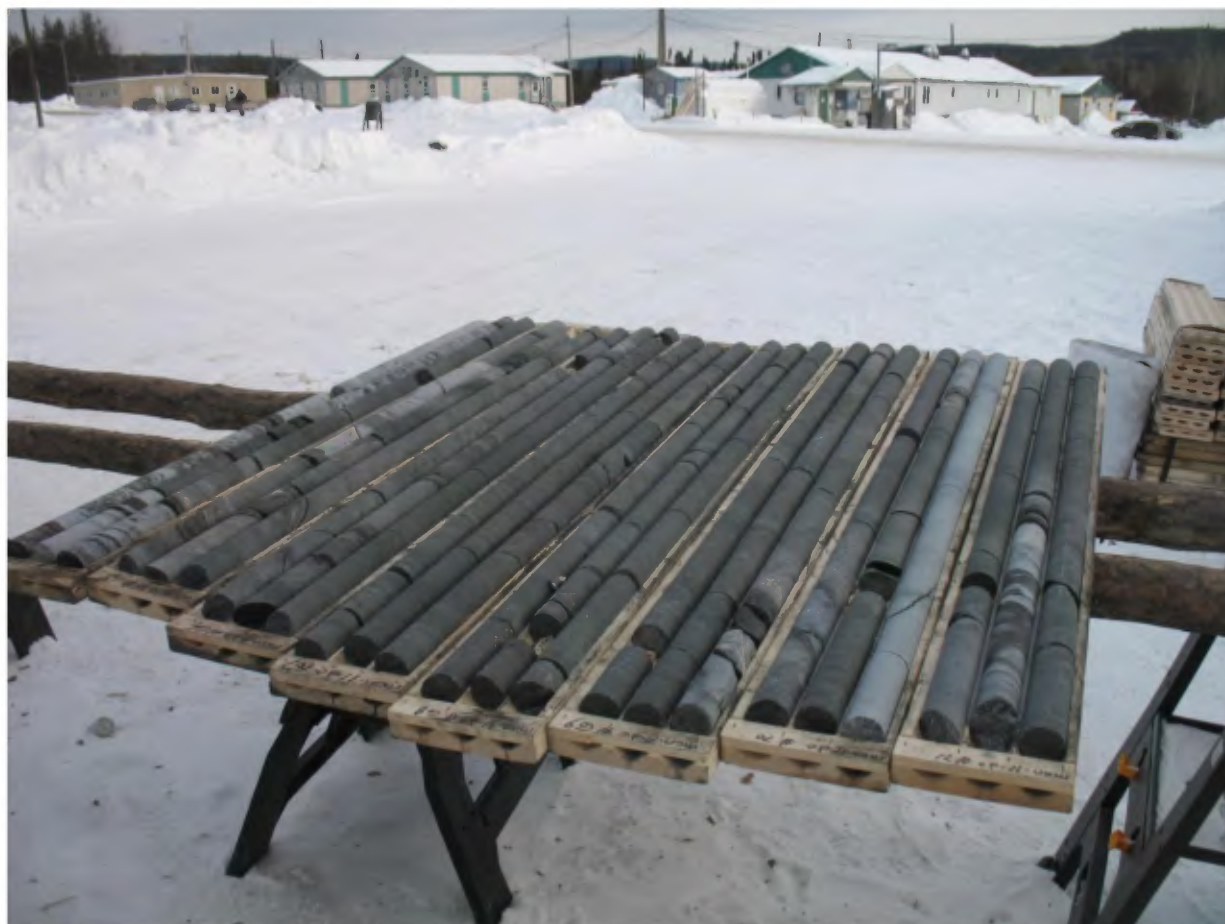
Photo 12.2 – Box opening and review prior to being logged
