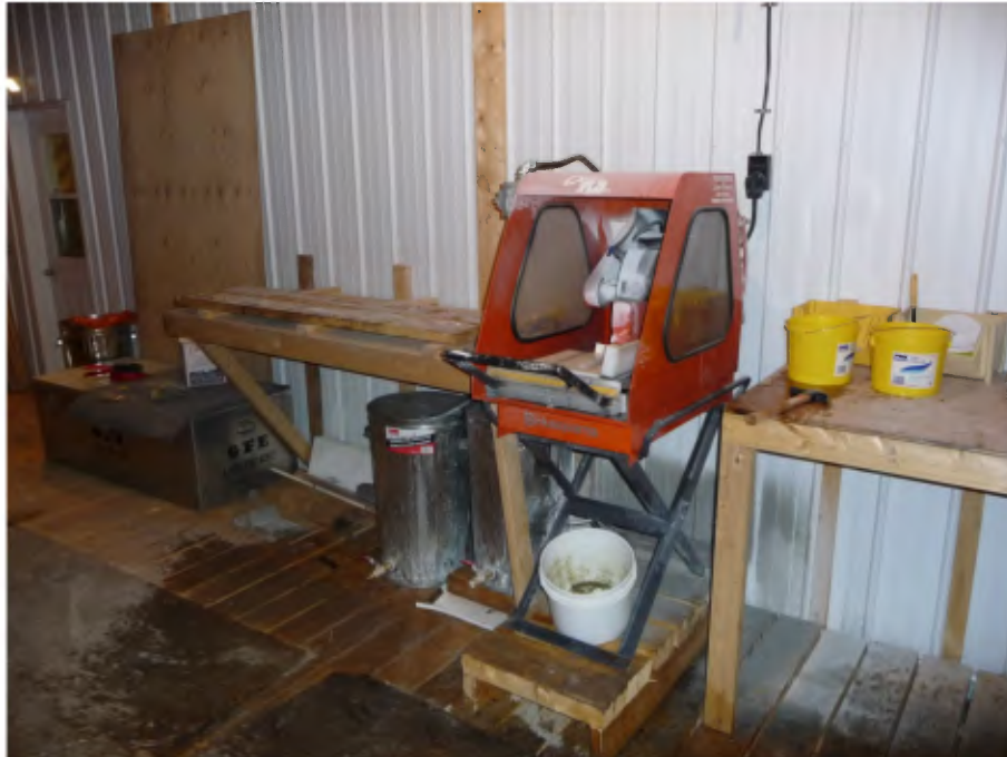
Core cutting and sampling facilities
