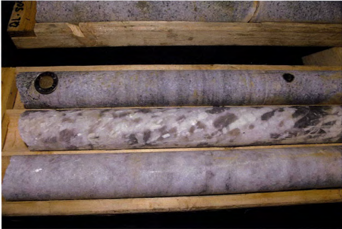
Figure 9- 2 Photograph of oriented green spodumene (comb structure) with interstitial quartz and aplite in drill core (middle of tray) from the Quebec Lithium Property. Coin for scale is 2.8 cm in diameter.
