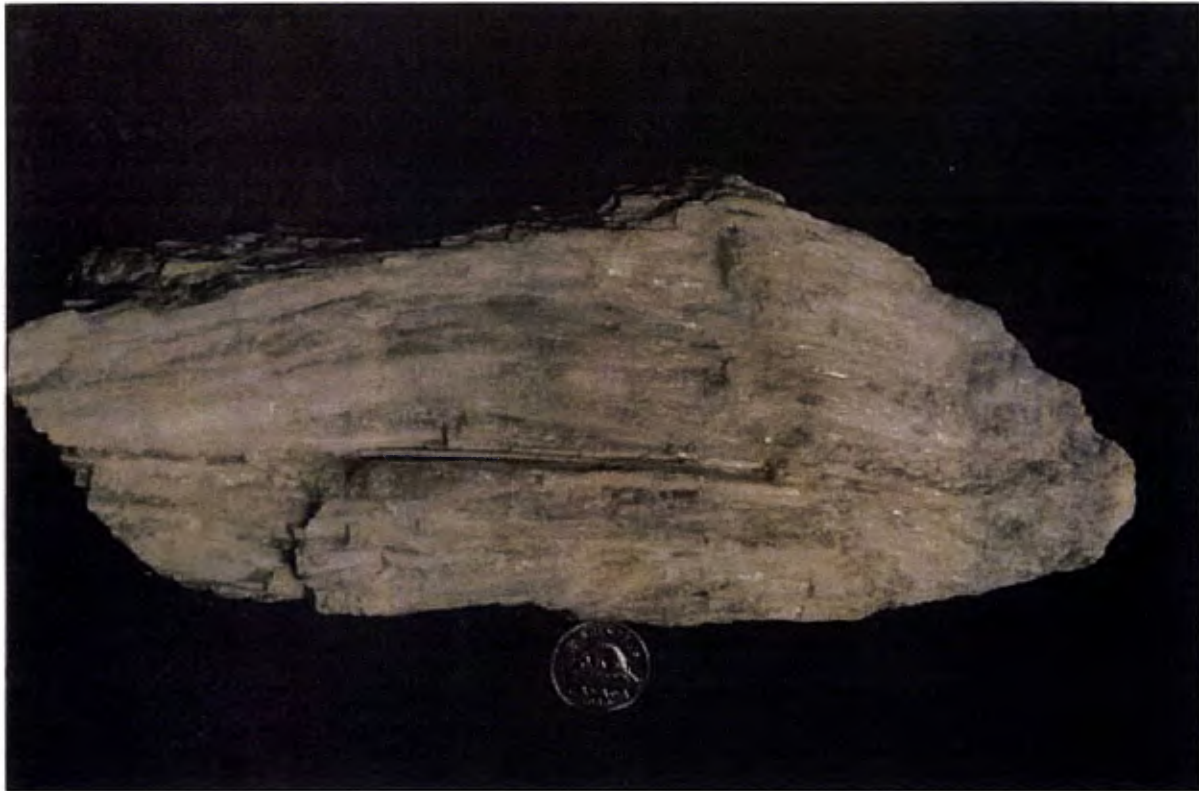
Figure 4- 3 Photograph of spodumene (elongate mineral)-bearing pegmatite from Dyke B at the Quebec Lithium mine (Karpoff, 1993). Coin for scale is 21.2 mm in diameter.
