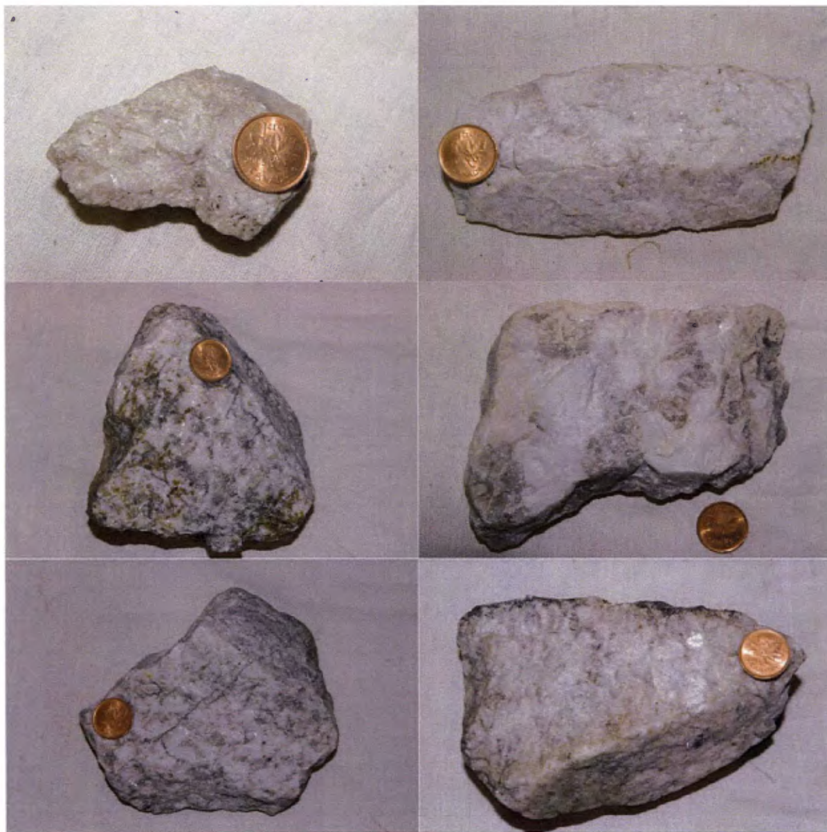
Figure 14- 3 Photographs of the rock samples collected to form the composite for geochemical analysis. Penny for scale is 19.05 mm in diameter.
