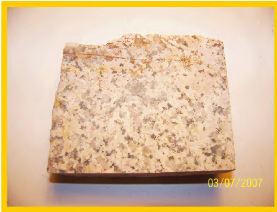
Figure 8a. Sample POCH10. Poularies tonalite. Note the absence of yellow staining in rock testifying to the absence of potassic feldspar. UTM Coord; Easting: 645443; Northing: 5388130; NAD83; Zone 17N.
