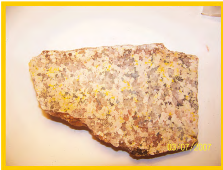
Figure 8b. Sample POCH01. Poularies tonalite. Note the paucity of yellow staining in rock (~ 1-2%) testifying to the rarity of potassic feldspar. UTM Coord.; Easting: 645446; Northing: 5388097; NAD83; Zone 17N
