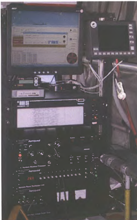
Figure 9. AeroTEM II Instrument Rack., including AeroDAS and RMS DGR-33 systems, AeroTEM power supply, data acquisition computer and AG-NAV2 navigation system.
