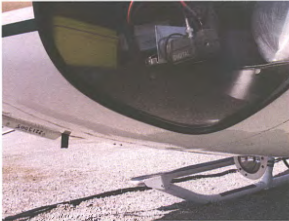
Figure 10. Digital video camera typical mounting location.
