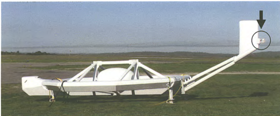
Figure 6. AeroTEM II EM bird. Arrow indicates the location of the second caesium magnetometer sensor.
