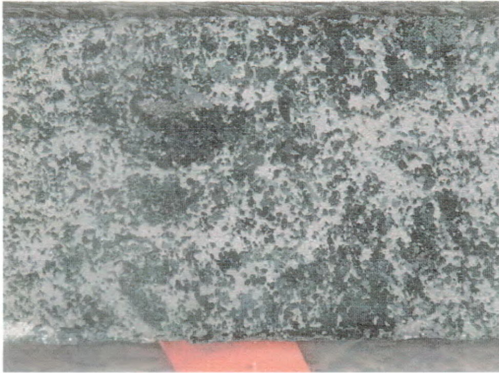
Figure 58 (H3-21). Amphibole- and pyrrhotite-rich part of relatively sulphide-rich section of quartzofeldspathic gneiss, 348-351 metres, DDHBQ03; wet, note scattered garnet and blebs of magnetite; core is 4 cm across in short direction.
