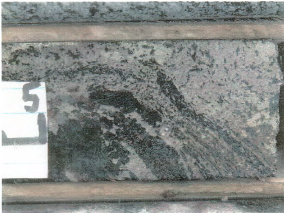
Figure 40 (H3-3). Pyrrhotite-, pyrite-, and amphibole-rich magnetite garnet biotite amphibole quartzofeldspathic gneiss; approximately 194-195 metres, DDHBQ03.
