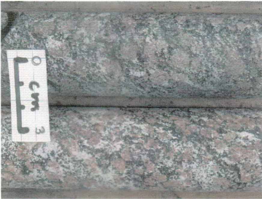
Figure 78 (H7-1). Relatively abundant garnet within (biotite) amphibole quartzofeldspathic gneiss; 75-80 metres, DDHBQ07.
