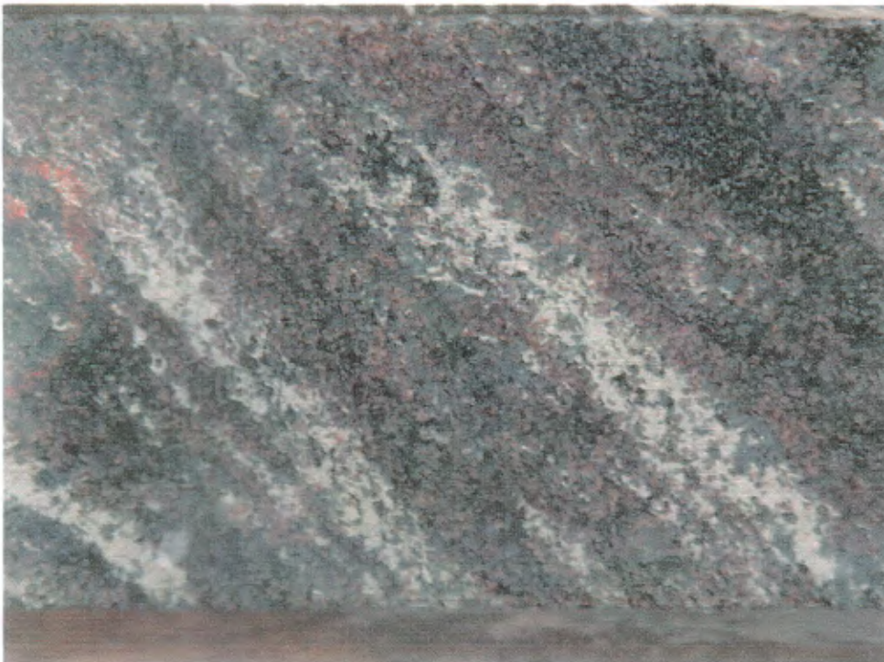
Figure 55 (H3-18). Well-layered pyrite- and garnet-rich quartzofeldspathic gneiss, 348-351 metres, DDHBQ03; core is 4 cm across in short direction.
