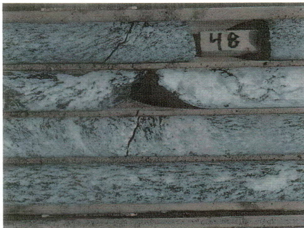
Figure 36. (H2-3). Fine-grained, well foliated and moderately well layered quartzofeldspathic gneiss, with abundant pyrrhotite and subordinate pyrite in close association with dark green amphibole and rare garnet and magnetite; 86 to 99 metres, hole DDHBQ02.
