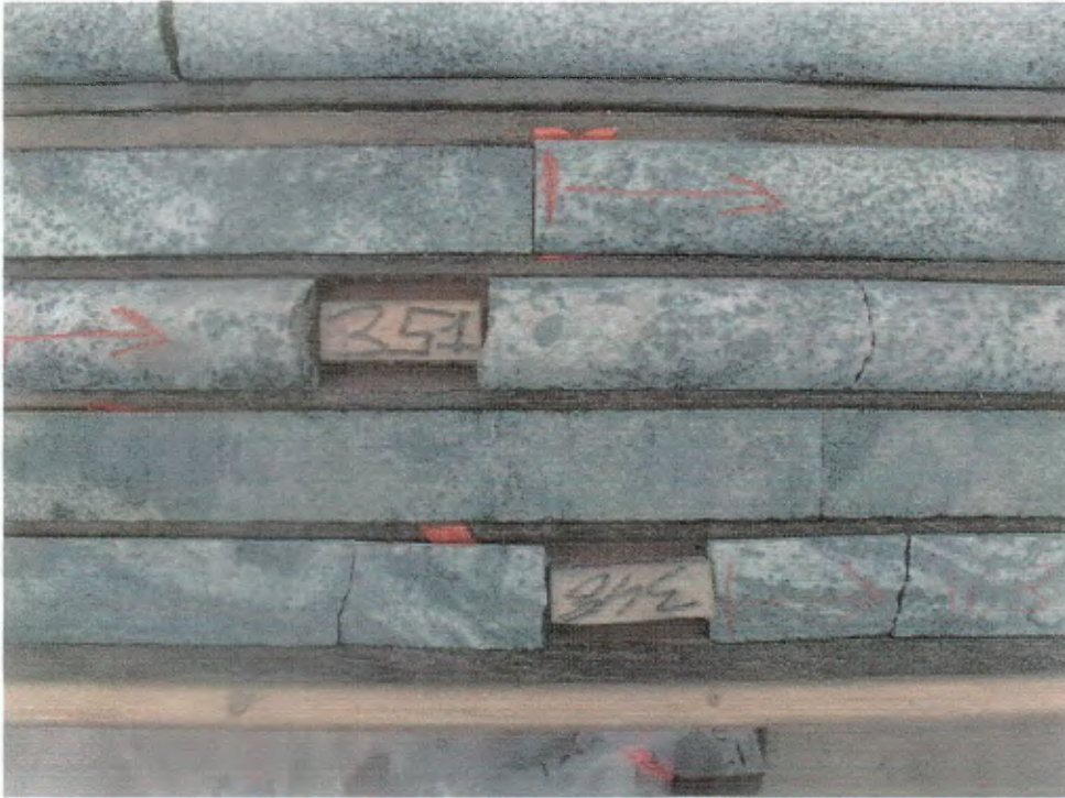
Figure 54 (H3-17). Mineralogically and texturally variable, relatively sulphide-rich section within quartzofeldspathic gneiss, 348-351 metres, DDHBQ03.
