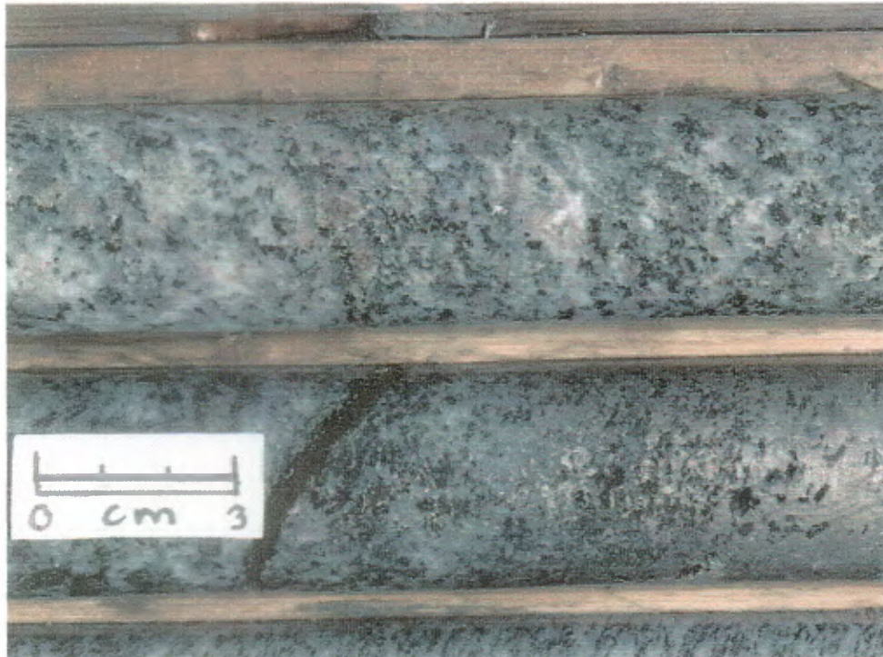
Figure 84 (H8-3). Disseminated to massive pyrrhotite and pyrite within garnetiferous biotite amphibole quartzofeldspathic rocks; 246-249 metres, DDHBQ08.
