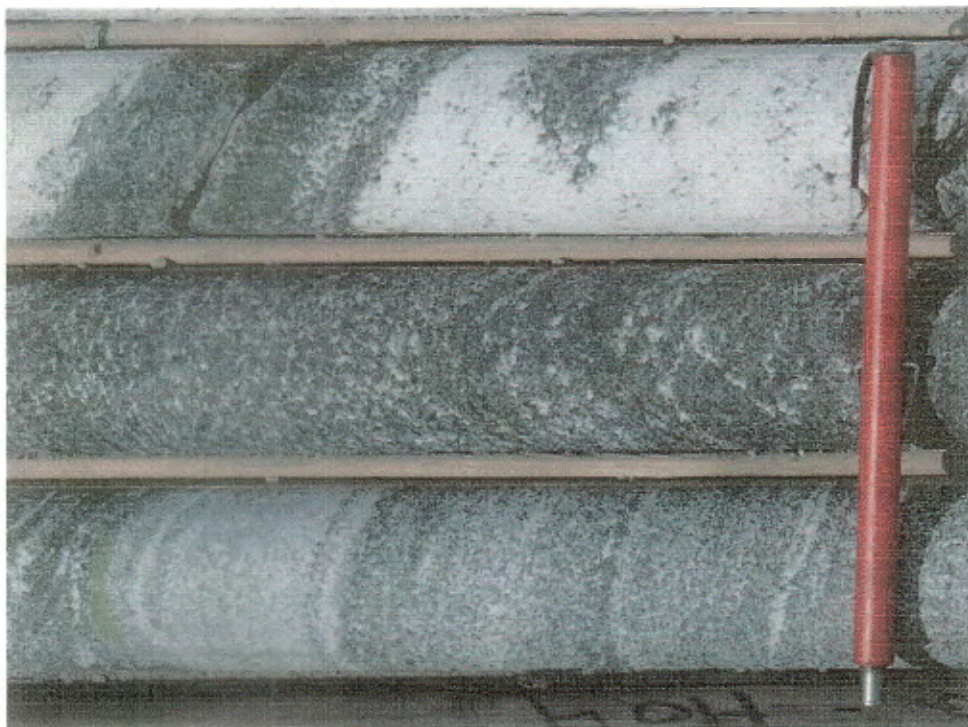
Figure 63 (H4-3). Well-layered amphibolite intruded by local (upper row) leucocratic granitoid rocks; 50-52 metres, DDHBQ04.
