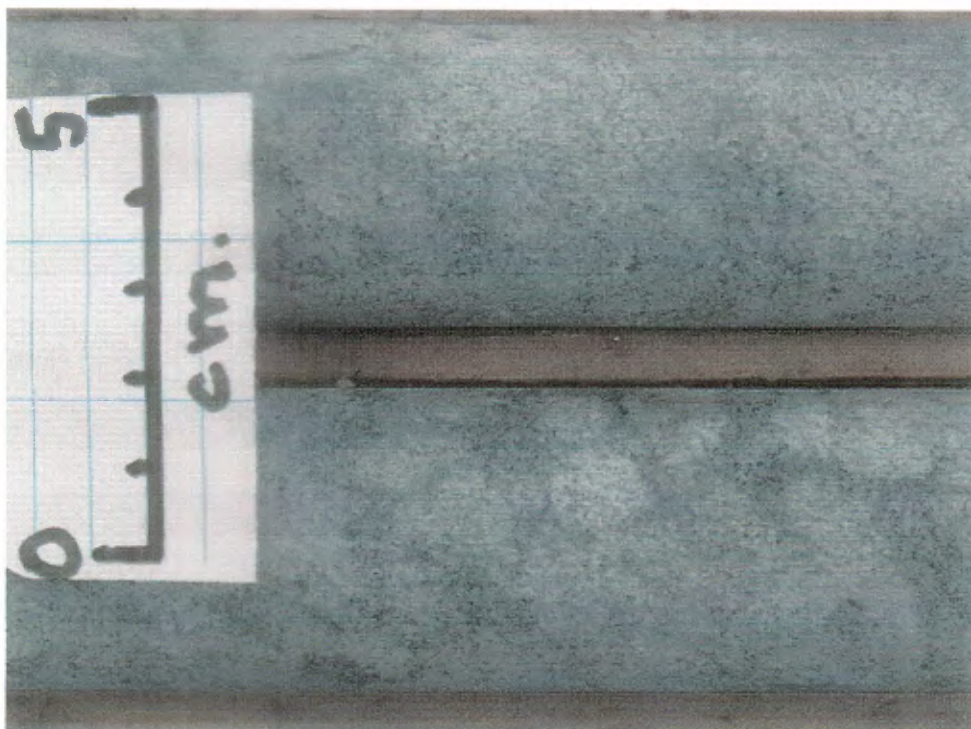
Figure 45 (H3-8). Nonfoliated amphibolite, 330-331 metres, DDHBQ03; pale coloured parts of mottled pale- to medium-green rocks represent crystallographically continuous amphibole which may be pseudomorphing poikilitic pyroxene.
