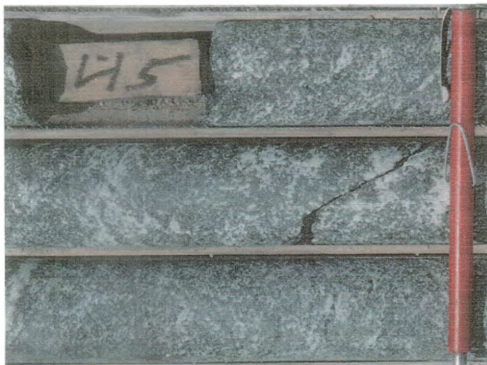
Figure 62 (H4-2). Fine- to medium-grained, dark green biotite amphibolite with a weakly developed foliation and weak magnetic character; 45-50 metres, DDHBQ04.
