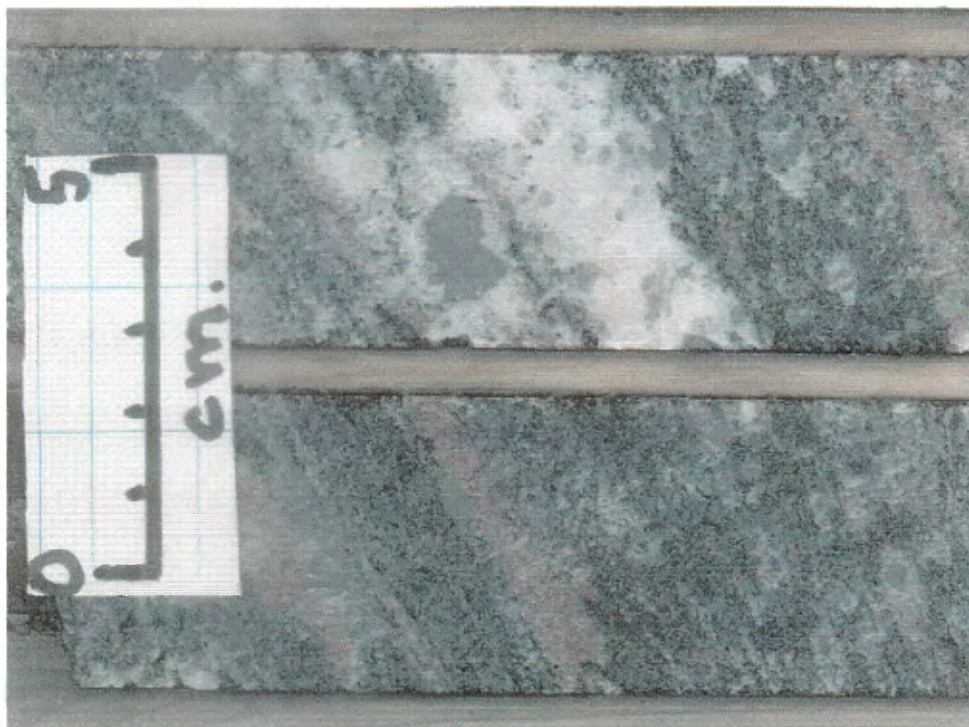
Figure 52 (H3-15). Slabbed pyrite garnet magnetite biotite quartzofeldspathic gneiss, 359-360 metres, DDHBQ03.
