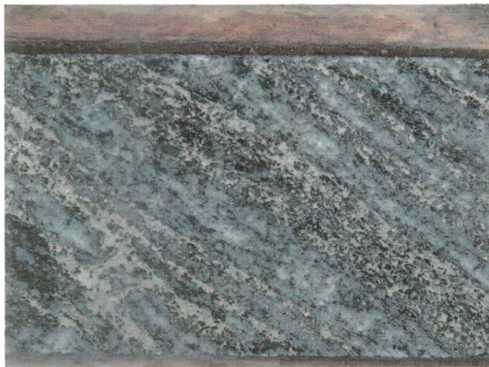
Figure 57 (H3-20). Well-layered pyrite-rich (plus magnetite) part of relatively sulphide-rich section of quartzofeldspathic gneiss, 348-351 metres, DDHBQ03; core is 4 cm across in short direction.
