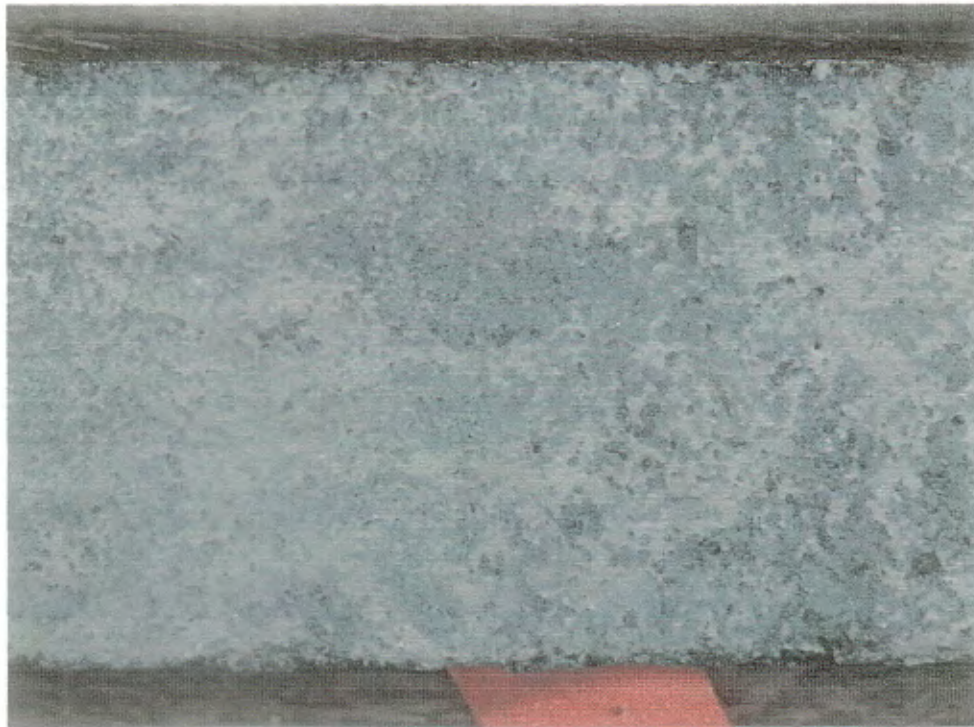
Figure 59 (H3-22). Amphibole- and pyrrhotite-rich part of relatively sulphide-rich section of quartzofeldspathic gneiss, 348-351 metres, DDHBQ03; dry; core is 4 cm across in short direction.
