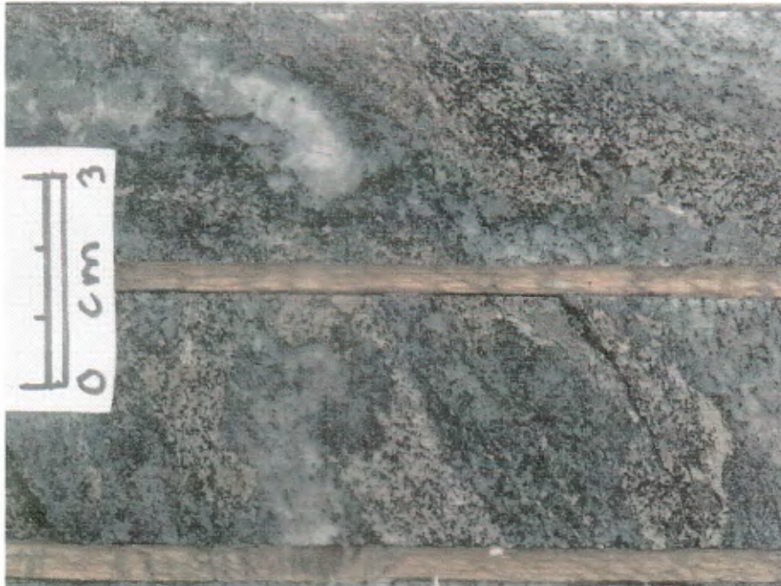
Figure 67. Heavily disseminated pyrrhotite and pyrite within garnet amphibole biotite quartzofeldspathic gneiss; approximately 127 metres, DDHBQ05.
