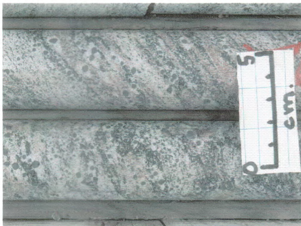
Figure 49 (H3-12). Biotite magnetite garnet quartzofeldspathic gneiss, 359-360 metres, DDHBQ03; core is 4 cm across in short direction.
