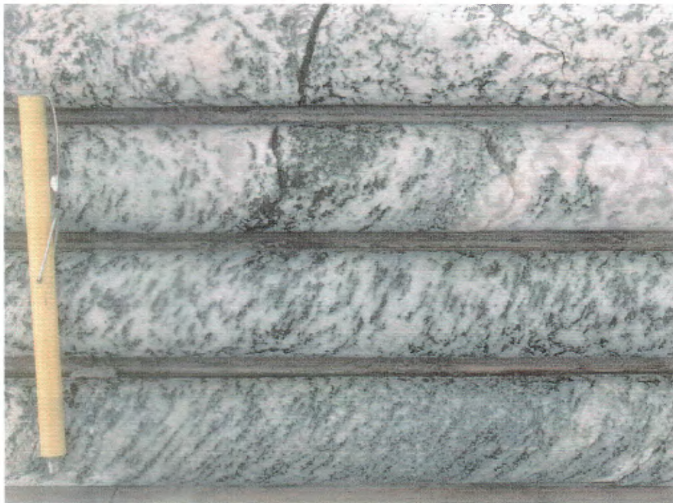
Figure 71 (H5-5). Well foliated biotite granodiorite, with local granite and granite pegmatite; approximately 190 metres, DDHBQ05.
