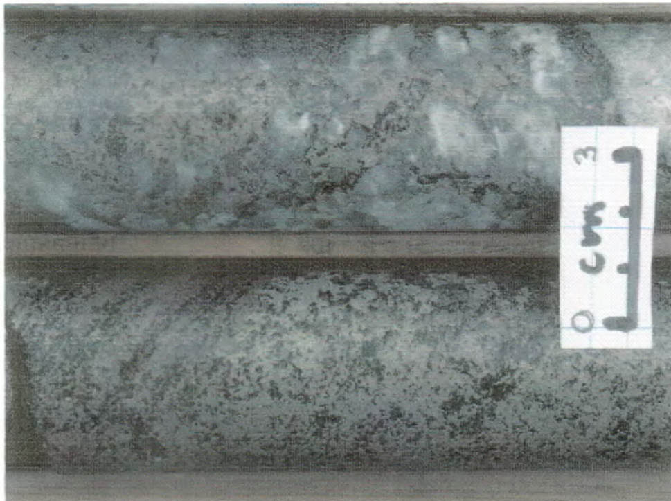
Figure 68 (H5-2). Semi-massive to massive sulphides in a host of garnet amphibole biotite quartzofeldspathic gneiss; 128-132 metres, DDHBQ05.
