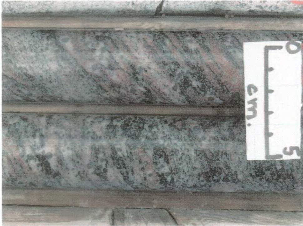
Figure 50 (H3-13). Biotite magnetite garnet quartzofeldspathic gneiss, 359-360 metres, DDHBQ03 (same as fig. H3-19, except wet; core is 4 cm across in short direction).
