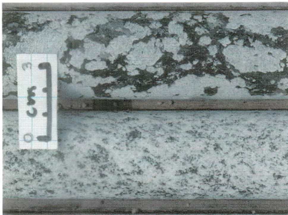
Figure 28. (H1-1). Gneissic granodiorite and biotite granite pegmatite (with minor pyrite) from the upper part of DDHBQ01; view is into foliation plane of gneissic granodiorite.
