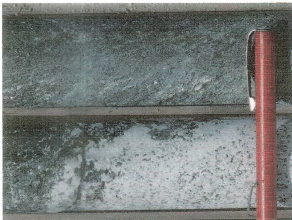
Figure 64 (H4-4). Detail of intrusive contact between dark green amphibolite of probable ultramafic origin and white gneissic granodiorite; from near the bottom of DDHBQ04.
