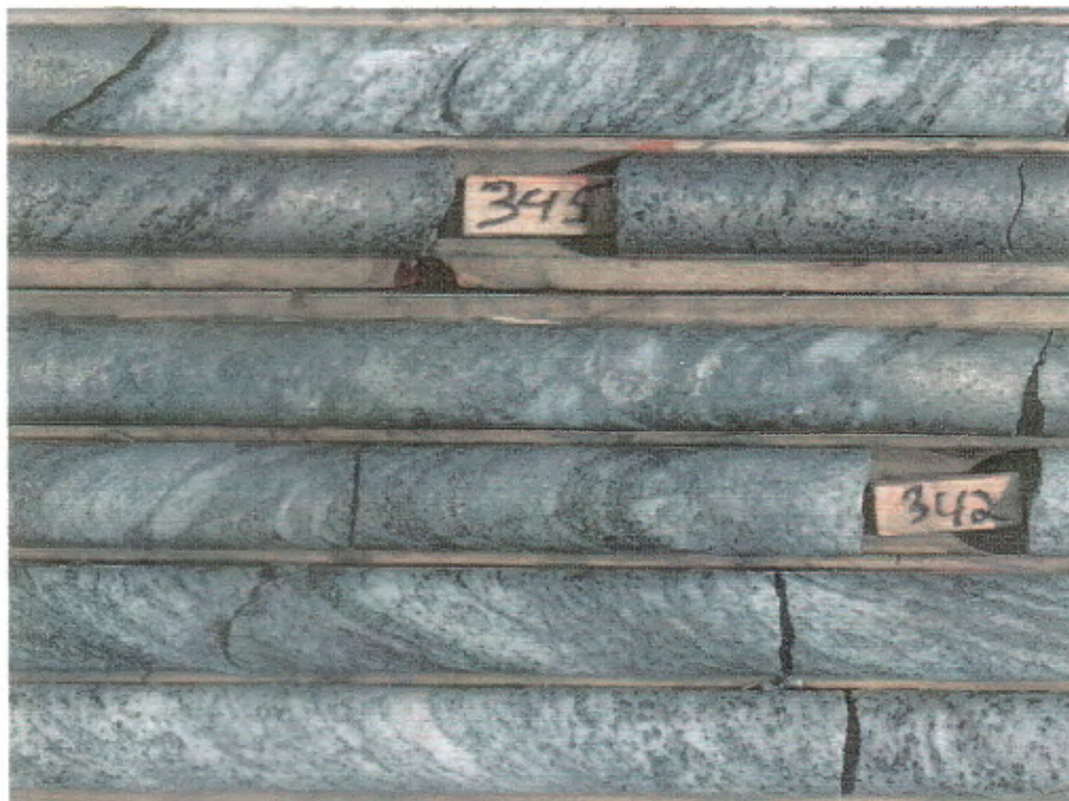
Figure 85 (H8-4). Section of relatively sulphide-rich paragneiss toward contact of gneissic granodiorite (leucocratic rocks in upper part of photo); from near bottom of DDHBQ08, 342-345 metres.
