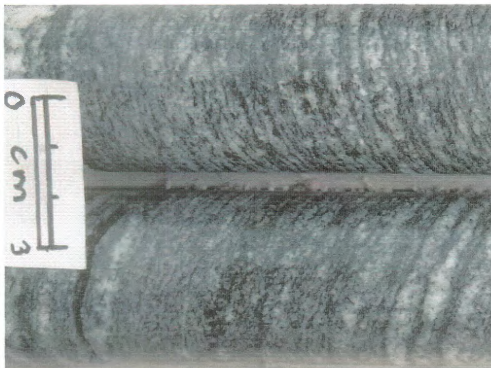
Figure 69 (H5-3). Well-layered, relatively biotite-rich garnet biotite quartzofeldspathic gneiss; 159-162 metres, DDHBQ05.
