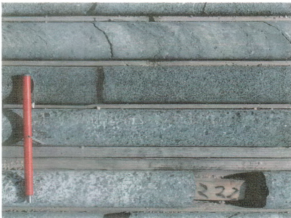
Figure 42 (H3-5). Variably foliated (biotite) amphibolites, 222-224 metres, DDHBQ03; amphibole pseudomorphs pyroxene in what were most likely feldspathic pyroxenites (bottom), pyroxenites, and more well-foliated peridotites (top).
