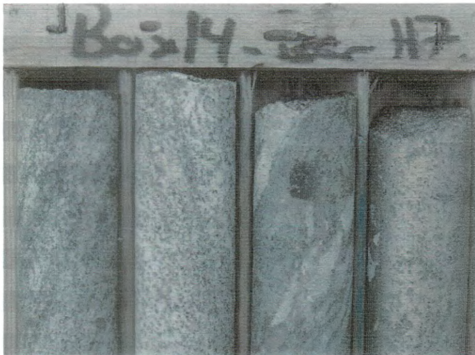
Figure 79 (H7-2). Typical mineralogical variation within interval of relatively sulphide-rich quartzofeldspathic paragneiss—note massive pyrrhotite in right-hand piece of core; 80-85 metres, DDHBQ07.
