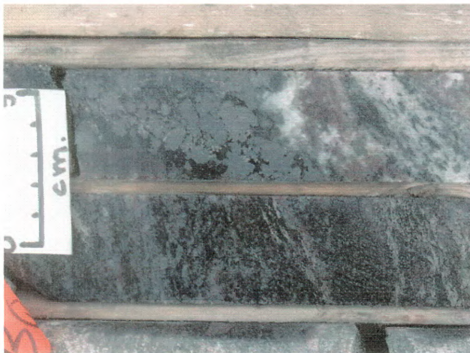
Figure 53 (H3-16). Slabbed pyrite garnet magnetite biotite quartzofeldspathic gneiss, 359-360 metres, DDHBQ03.
