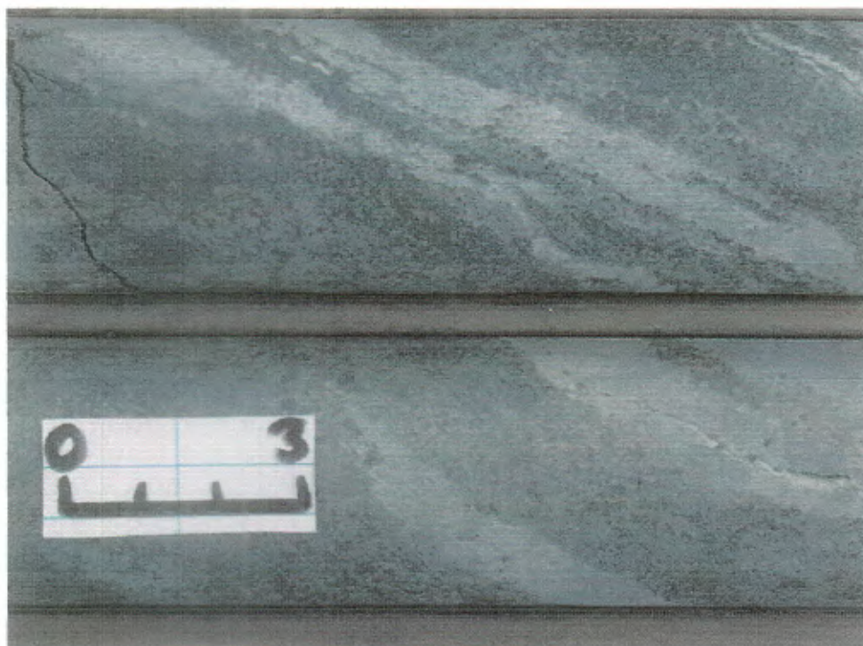
Figure 80 (H7-3). Relatively amphibole- and sulphide-rich paragneiss interlayered with leucocratic quartzofeldspathic layers; DDHBQ07.
