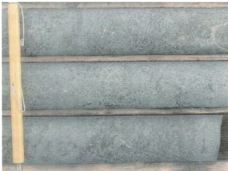
Figure 74 (H6-2). Magnetite biotite amphibolite typical of upper part of DDHBQ06.
