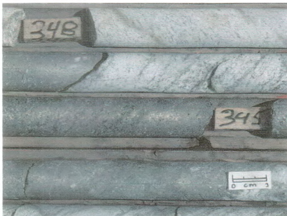
Figure 87 (H8-6). Detail of massive sulphides; from near bottom of DDHBQ08, 345-346 metres.
