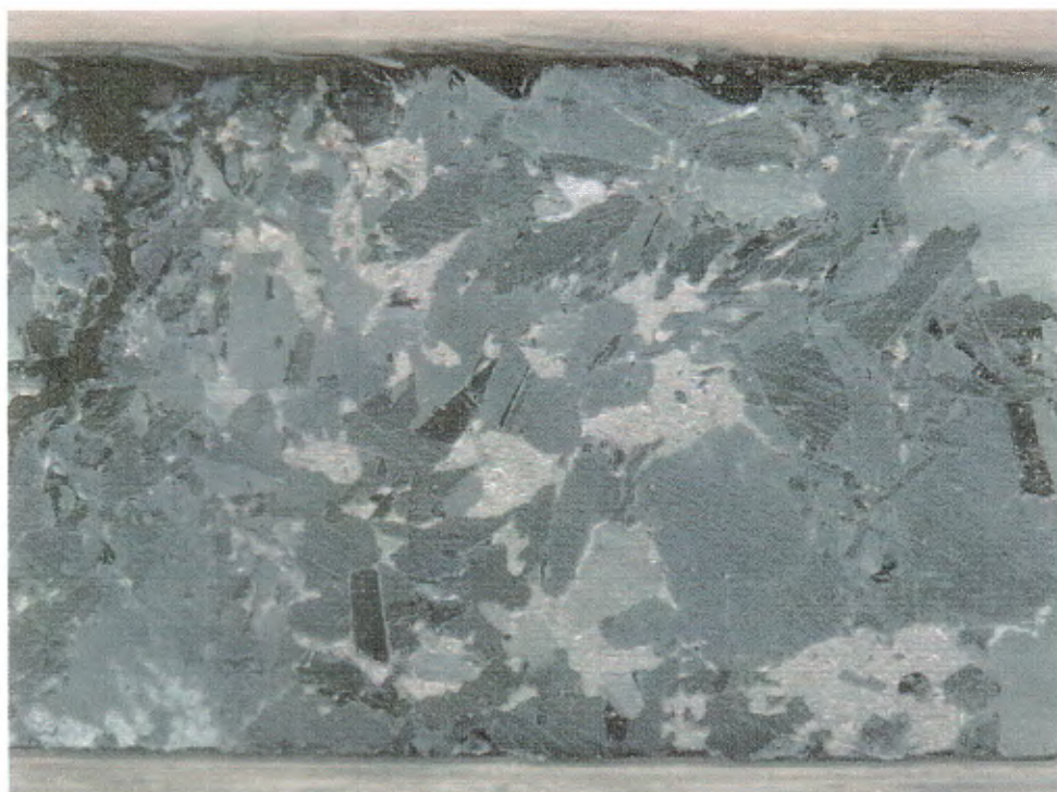
Figure 47 (H3-10). Biotite-rich part of pyrrhotite (pyrite) biotite granite pegmatite; approximately 337 metres, DDHBQ03; note specks of chalcopyrite in upper part of slabbed core; core is 4 cm across in short direction.
