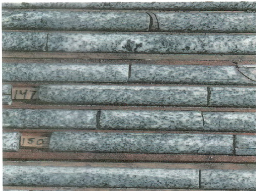
Figure 31 (H1-4). "Spotted" gneissic granodiorite of interval from which blank samples were collected, approximately 143-152 metres, DDHBQ01.
