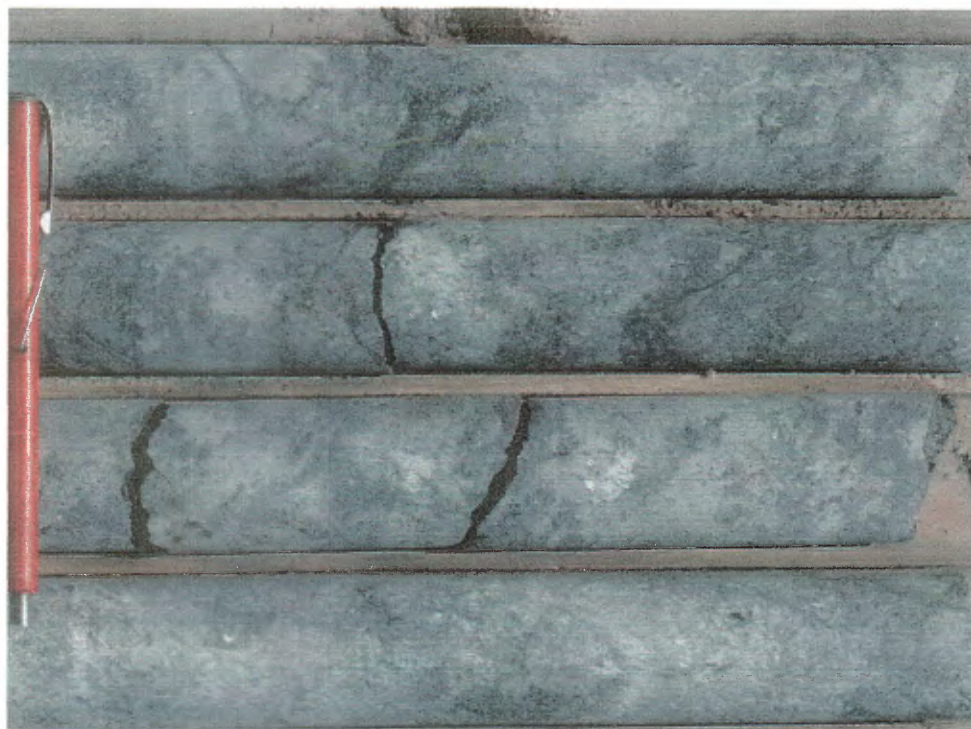
Figure 44 (H3-7). Nonfoliated coarse-grained amphibolite, 330-331 metres, DDHBQ03; very coarse-grained, crystallographically continuous amphiboles may be pseudomorphs after poikilitic pyroxene.
