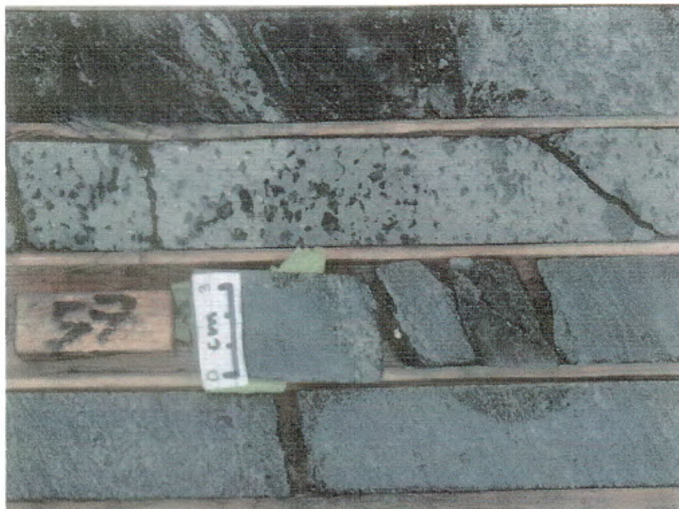
Figure 82 (H8-1). Heavily disseminated, semi-massive, and massive pyrrhotite and pyrite within amphibole-rich paragneiss; 57-58 metres, DDHBQ08.
