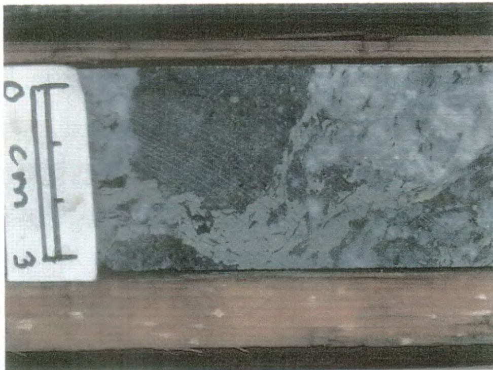
Figure 30 (H1-3). Pegmatite-hosted pyrite mineralization, DDHBQ01.
