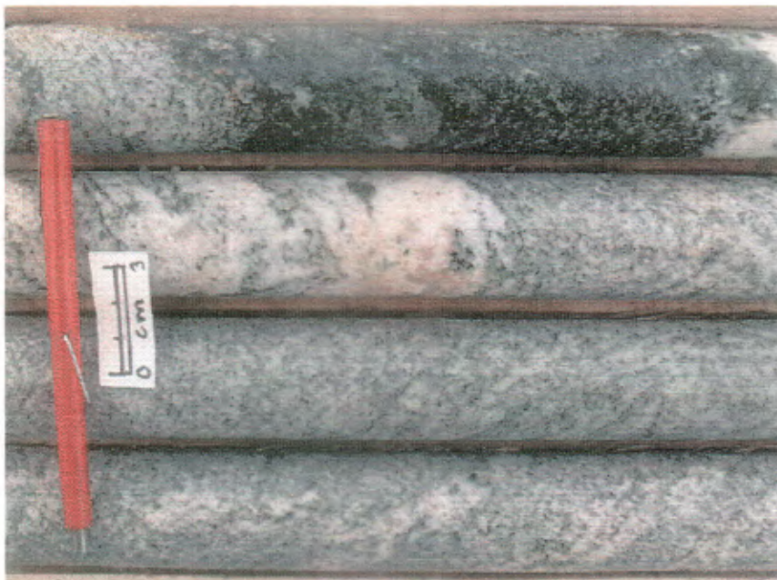
Figure 34.(H2-1). Core from the uppermost 10 metres of DDHBQ02, showing predominant biotite granodiorite gneiss and subordinate medium to dark green biotite amphibolite (top), and white to pink granite.
