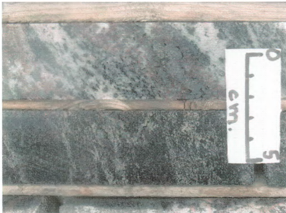
Figure 51 (H3-14). Pyritic magnetite biotite garnet biotite quartzofeldspathic gneiss, 359-360 metres, DDHBQ03.
