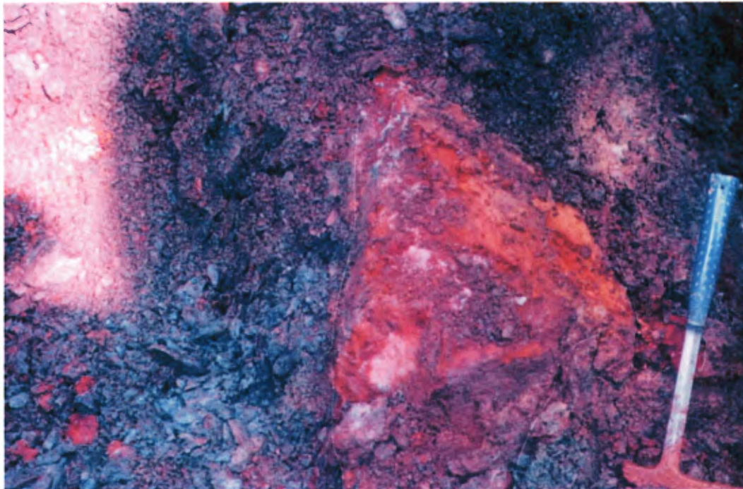
PHOTO 7A - Close Up Of Donat Carbonate, Chlorite, Shear With Oxidized Sulphide Clasts
