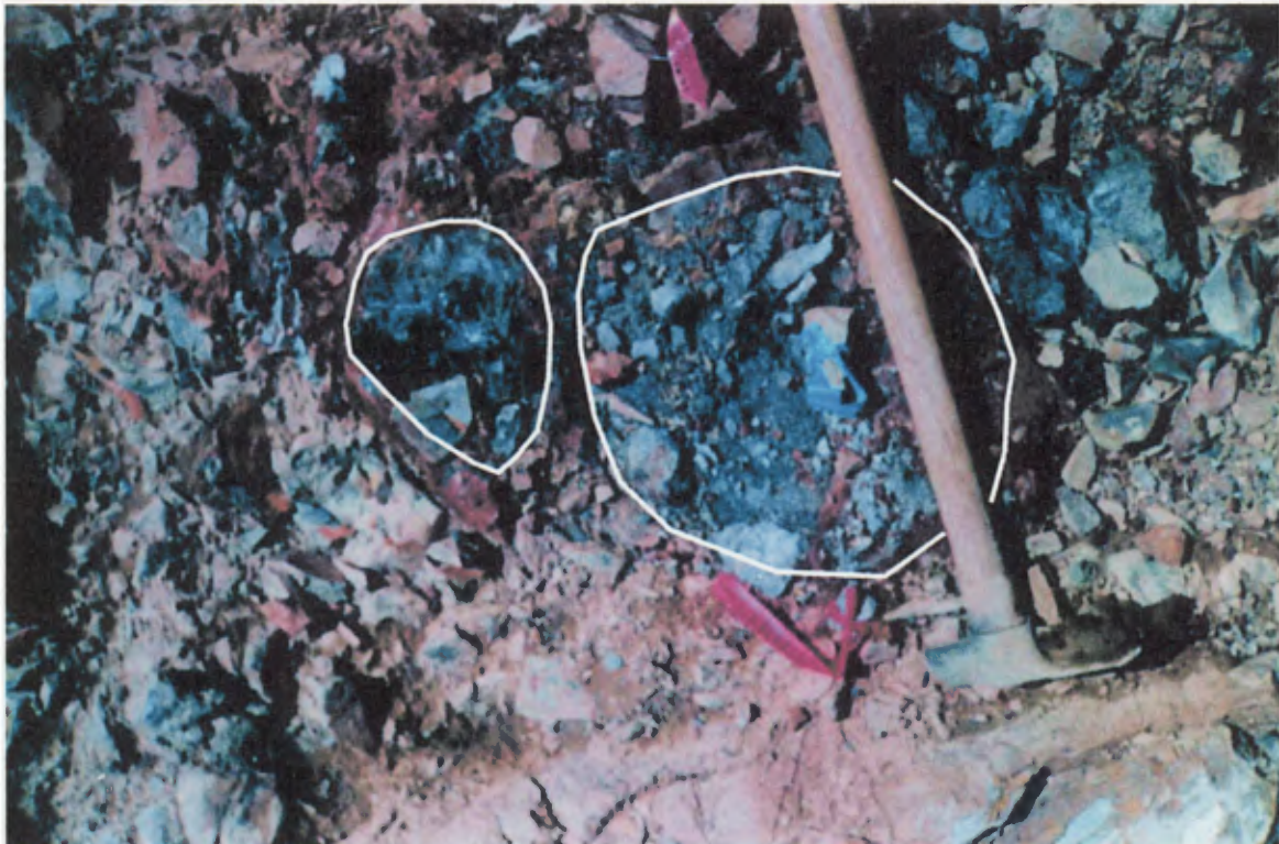
PHOTO 2B- Close Up OF Mersereau Breccia - Massive Sulphide Clasts
