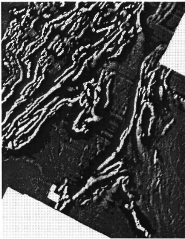
Figures 7 and 8. High gain AGC filter after CGI fix of GPS GTIME problem ( Figure 7 -left image) and after reprocessing from scratch (Figure 8 -right image). In Figure 7, the numerous glitches seen in Figure 6 have been removed but there are still clear parallax problems seen as pulls and kinks. In Figure 8 the parallax problems have been reduced and line to line correlation is improved.
