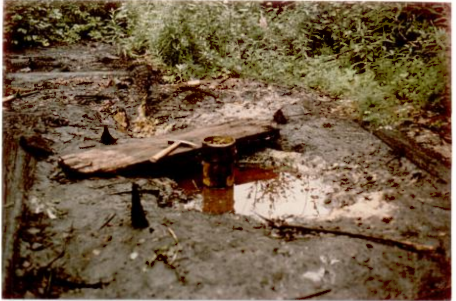
Photograph 1: POT 20, on road to Murdochville, 20 miles from Gaspé, flows 1/2 gallon of red waxy oil per day.
