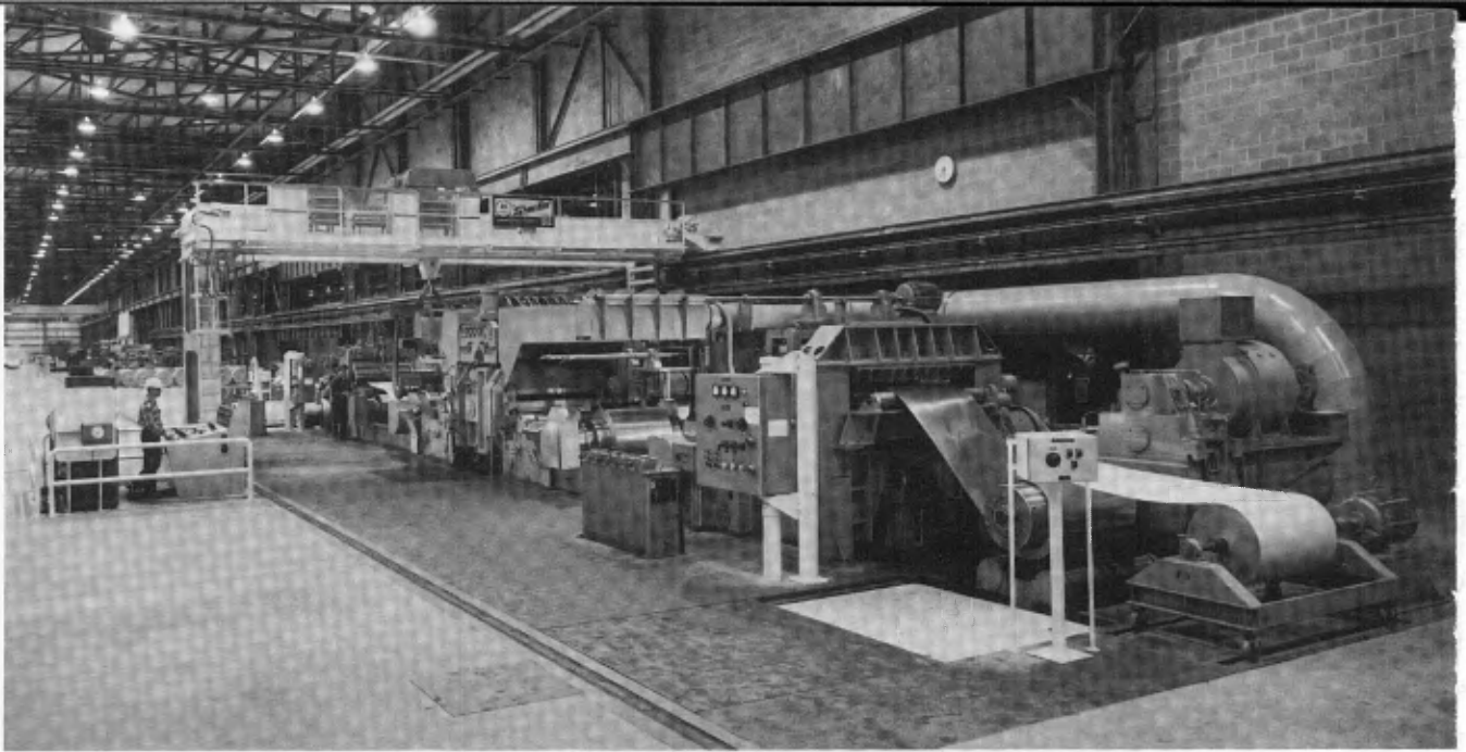
Computer-monitored Sendzimir cold rolling mill at Atlas Steels' Quebec plant reduces the thickness of 48-inch-wide, hot-rolled stainless steel coils down to industry standard sheet thicknesses.
