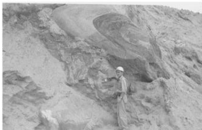
Kame deposit. Large boulders of folded gneiss (one above observer) in bedded fine sand. Stratification dips 35^{\circ} on top of boulder near feet of observer, lies sub-horizontal near his compass. Sand pit 1\frac{1}{2} mile west-northwest of Manic 2 dam.
