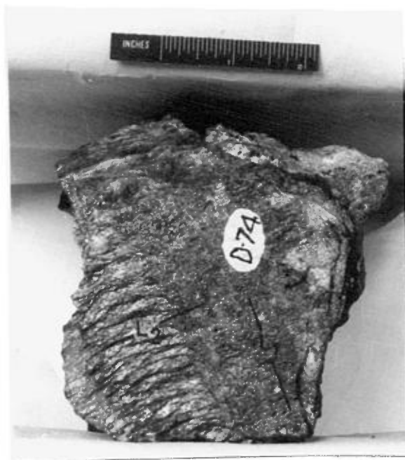
A. Bonsecours schist sample illustrating lineations L_1 and L_2 . Crinkles, associated with the later period of deformation, produce L_2 , sloping gently to the left. Quartz rods ( L_1 ), associated with the early folding, slope steeply to the right and apparently truncate L_2 . This is due to differential erosion, whereby the more resistant quartz rods, unaffected by crinkling, are preserved preferentially to the micaceous material. (in the vicinity of Eastray Station).
