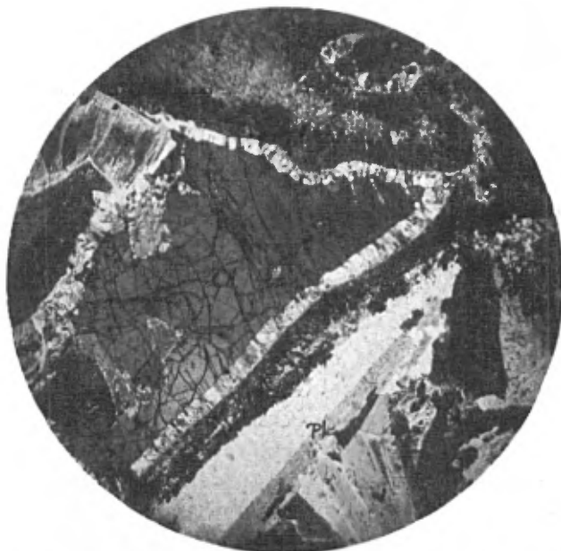
B- S-93-6. Photomicrograph, diameter 6mm. Crossed nicols. Coronitic gabbro. Rim of secondary pyroxene and garnet around olivine (Ol). Pl = plagioclase, Px = primary pyroxene.
