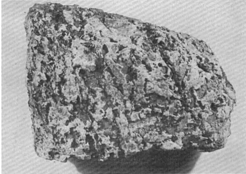
Nepheline syenite from the area north of the Obedjiwan Indian reservation. Note the microlitic texture.
