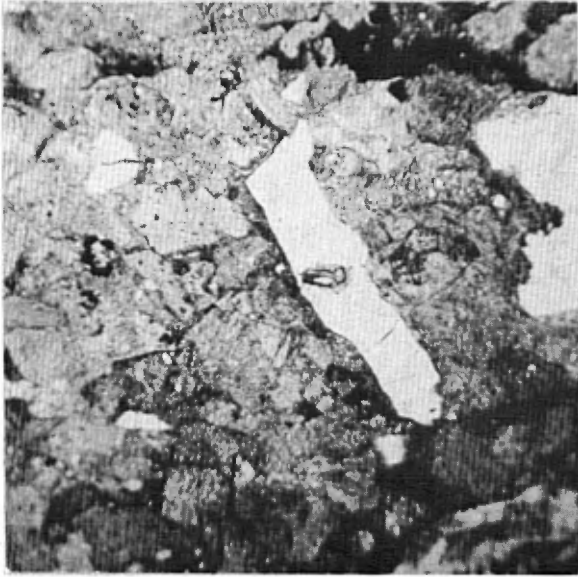
A.- Quartz crystal in porphyry conglomerate breccia. Note porphyry inclusion in middle of crystal Crossed nicols x 30.
