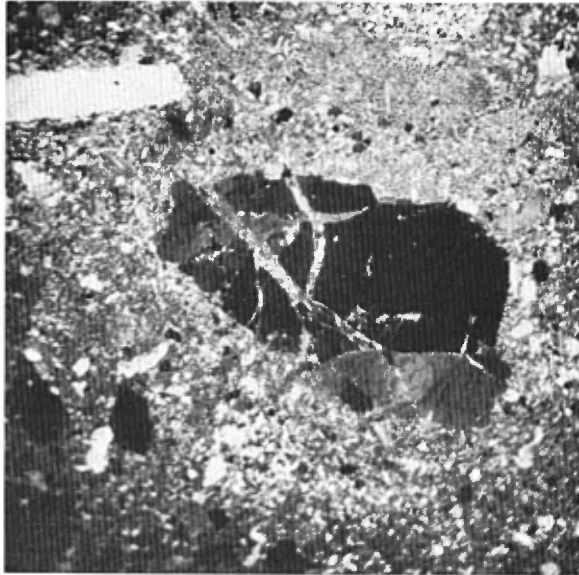
B.- Matrix of porphyry conglomerate breccia filling fractures in quartz phenocrysts. Crossed nicols x 15.
