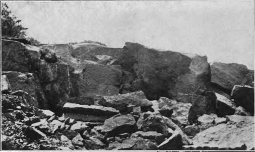
A.—Abandoned quarry of the Black Granite Co., Saint-Gédéon, showing the streaks in the stone and the character of the breaks.
