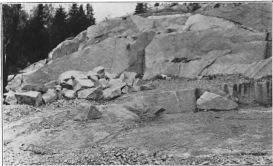
B.—South end of the Bernier quarry in Roberval granite, showing the slope of the sheets and their irregularity.
