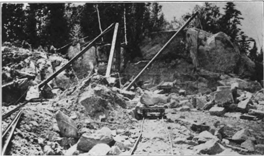
B.—Quarry of the National Granit Enrg., Saint-Gédéon, in black anorthosite. The rift structure may be seen dipping to the left back of the derrick's boom.
