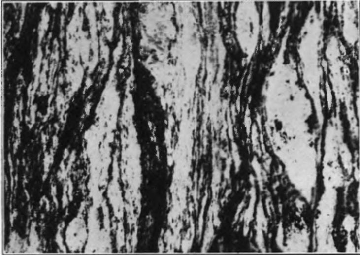
A.—Augen gneiss in rose and black developed from Roberval granite. Rocks of this texture are common in the Laurentian area and might be used for ornamental material.
