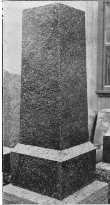
B.—Polished die with hammered base made from Roberval granite from Polycarpe Moreau quarry.
