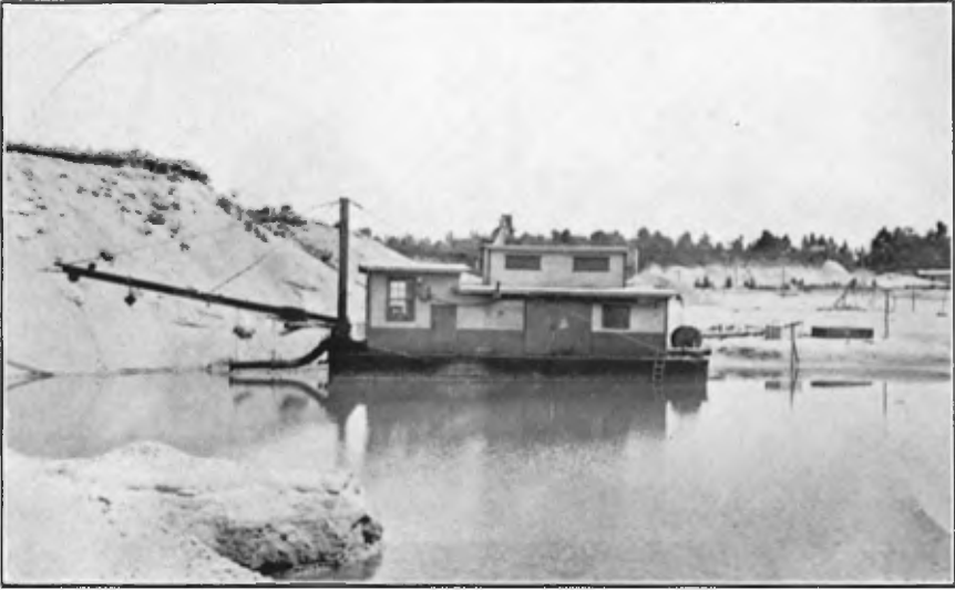
A.—Suction dredge in an artificial pond, at sand deposit of Standard Lime Company, Limited, St. Félix de Valois, Joliette county.
