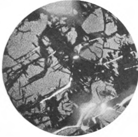
A.—Photomicrograph of chromite from Black Lake. The opaque portion, high in iron, sends off arms into the translucent reddish-brown substance (see p. 32) (From Dresser's Memoir 22, Geol. Surv. of Can.)
