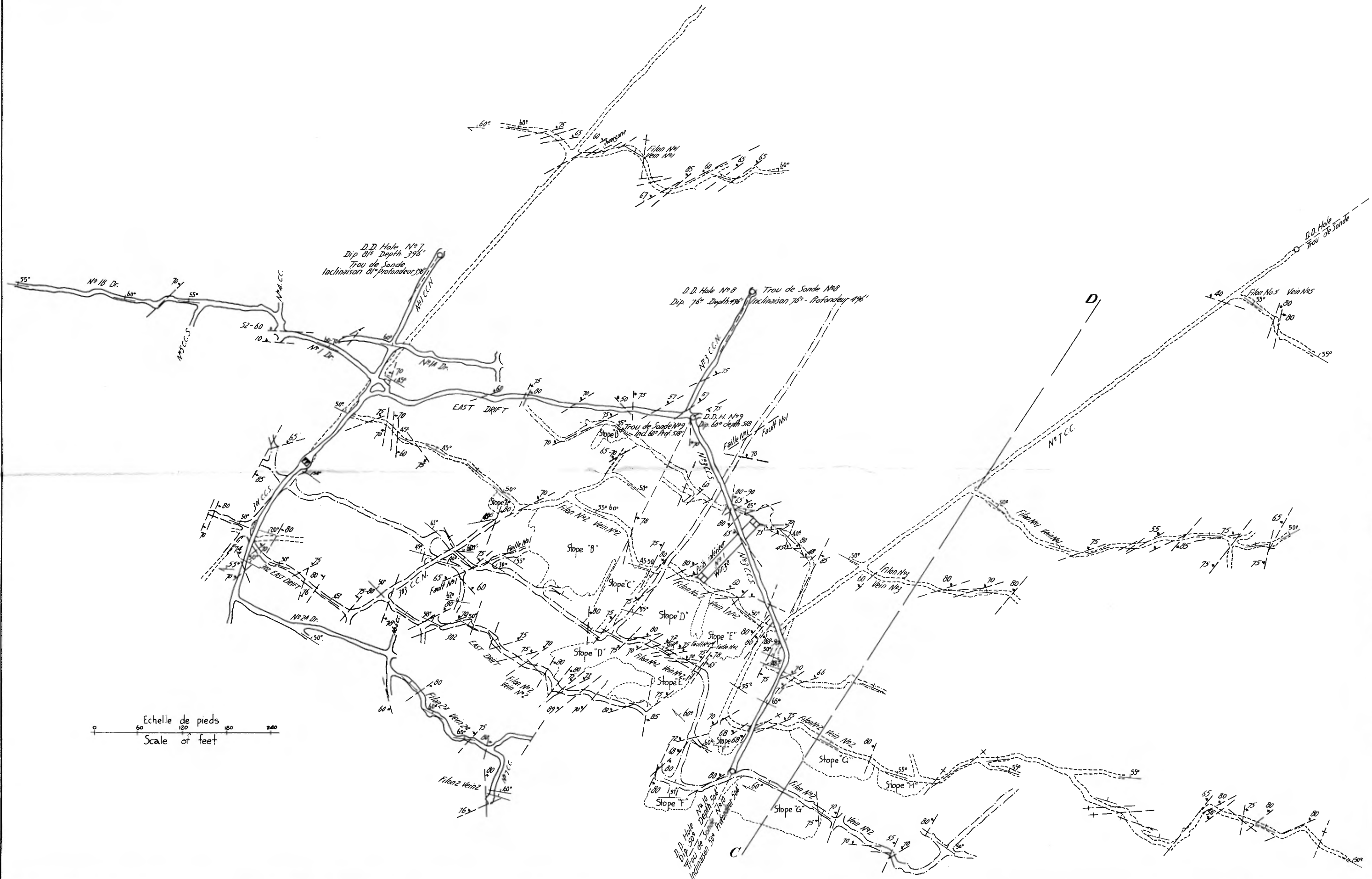
PLAN OF UNDERGROUND WORKINGS AT GRANADA MINE
