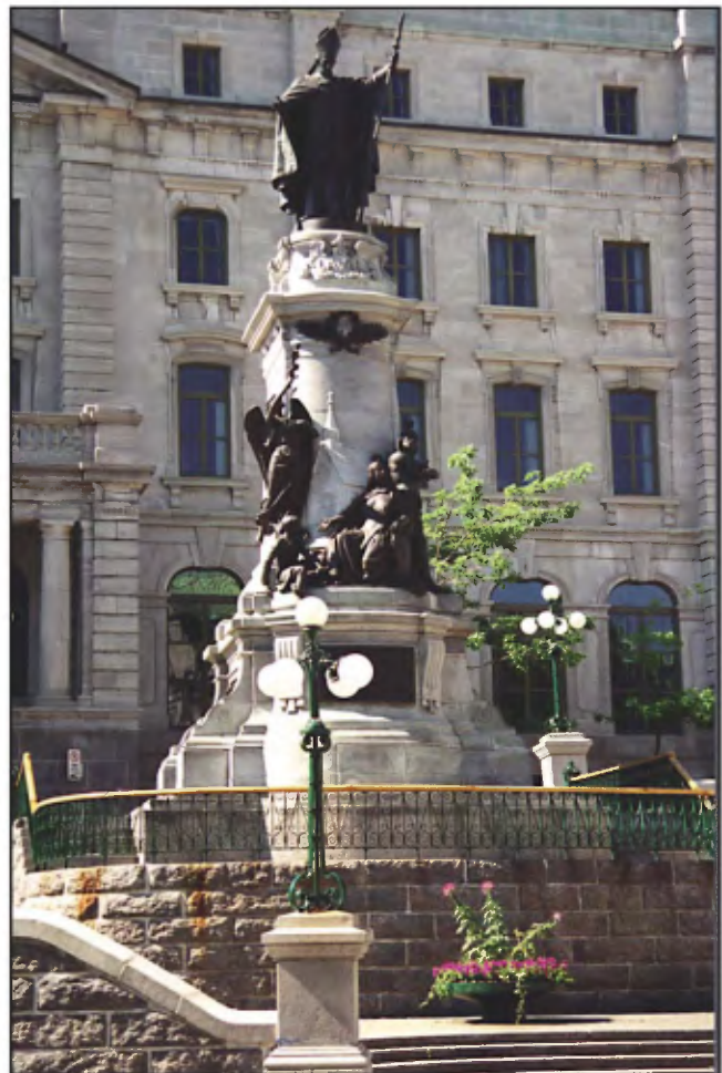
Monseigneur de Laval Monument with pedestal in Stanstead granite and ramp in Rivière-à-Pierre granite.
