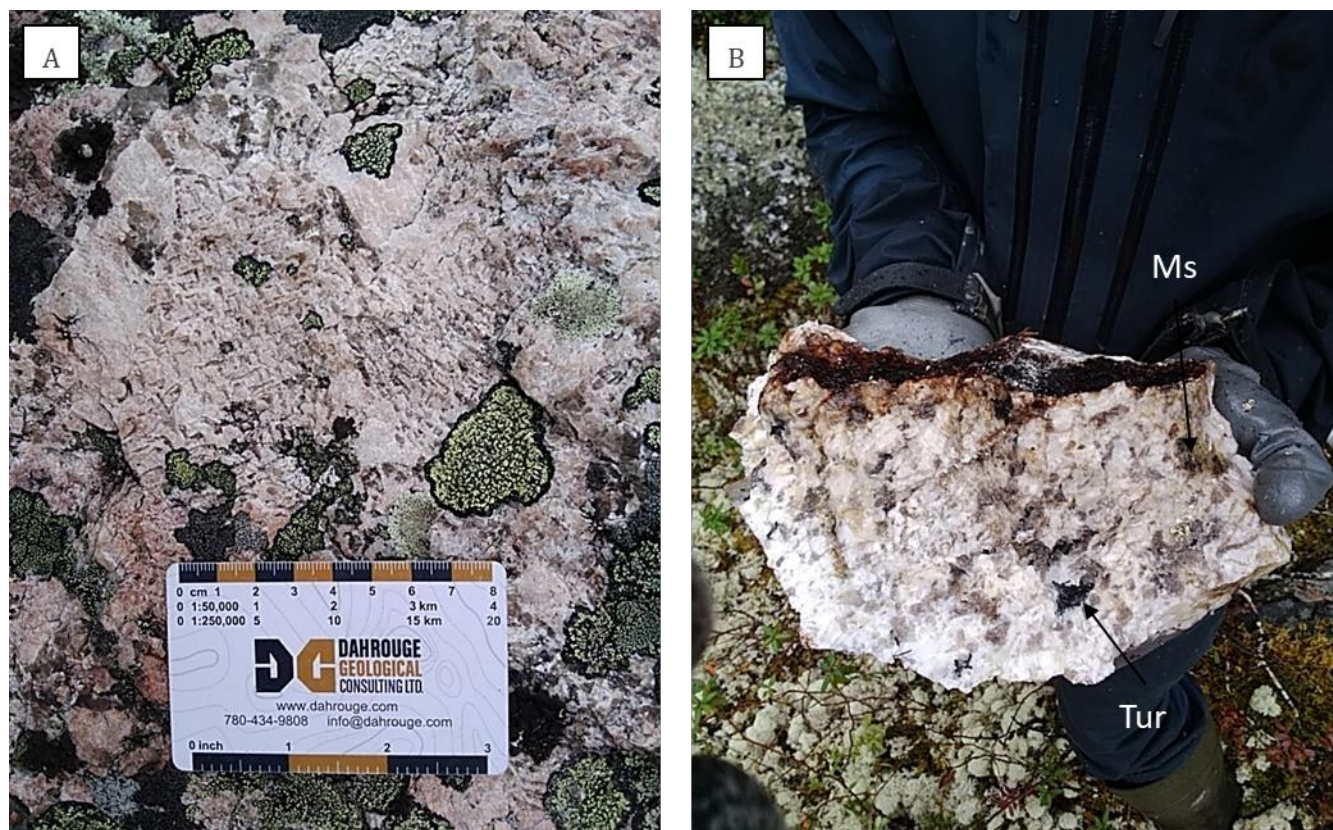
Figure 5-6 Boulder and boulder sample photos. A: Boulder of biotite bearing pegmatite with graphic texture from station NC23LGM-007. B: Sample C00430768, pegmatite with muscovite (Ms) and tourmaline (Tur) from station NC23LGM-015.
