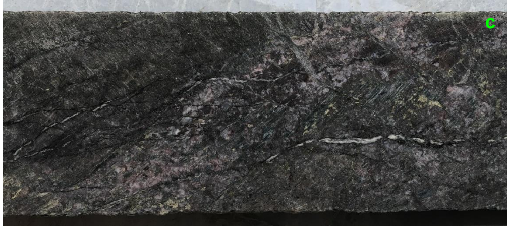
Figure 9. Photos of core from drillholes DO-20-275, DO-20-279 and DO-20-282 at Nika Zone, NQ-size (47.6 mm diameter), half-sawn.
