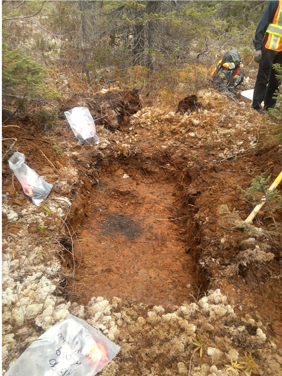
Photo 3: Example of sulphides occurrence in the PGE zone. Sulphides were found using a Beep Pap IV. Here, station 1418-21HL059 (samples 14189032@34). The dark spot is massive pyrrhotite.
