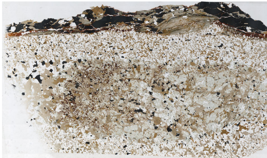
Figure 1: Thin section of sample 141890014 under natural light. The lighter part is quartz-rich, the greenish medium grey is actinolite-rich and the black edge is sulphide-rich vein.
