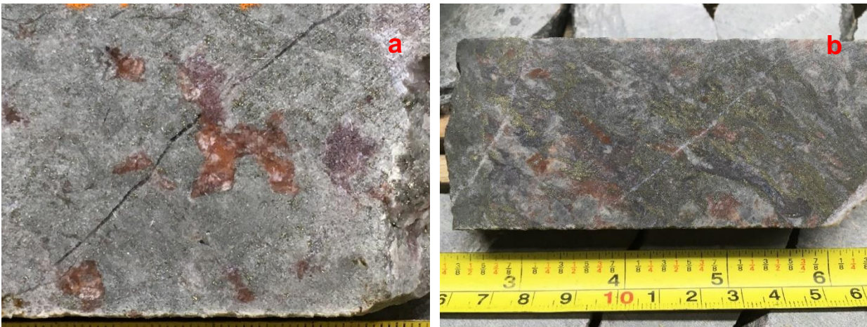
Figure 8. Photo of the core from drillhole DO-19-105X. Salmon pink Ca-carbonatite vein with brecciated fragments of carbonatized basalt; half-sawn NQ drill core (47.6 mm); 484.5-485.5 m @ 0.20 g/t Au.
