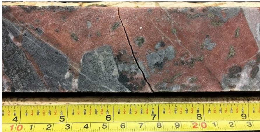
Figure 8. Photo of the core from drillhole DO-19-105X. Salmon pink Ca-carbonatite vein with brecciated fragments of carbonatized basalt; half-sawn NQ drill core (47.6 mm); 484.5-485.5 m @ 0.20 g/t Au.
