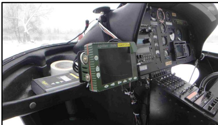
Figure 9 - AgNav navigation console mounted in helicopter.
