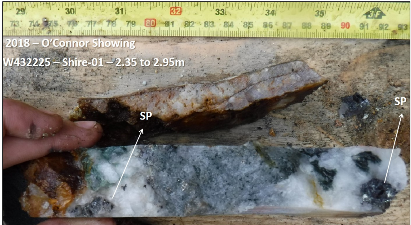
Figure 6. Sample W432225 on channel Shire-01. Best Zn value obtained in 2018. 2290ppm Zn over 60 centimeters.
