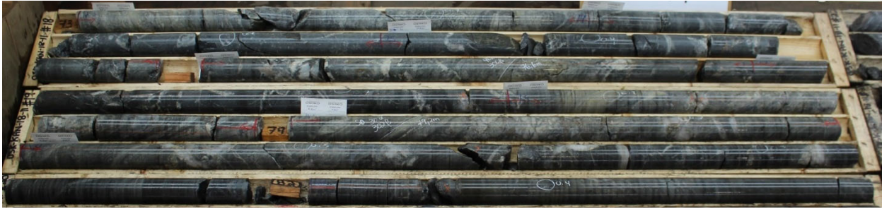
Photo 16: OSK-KAN-18-011 from 73 to 83 metres, Overview of the interval that returned 0.38 ppm Au over 5 metres from 77 to 82 metres.
