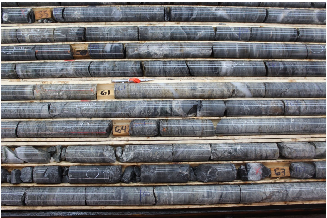
Photo 15: OSK-KAN-18-011 from 55 to 69 metres, Overview of the bleaching, as well as ankerite-chlorite-sericite penetrative alteration in carbonate iron formation found in the hinge zone of the Ferricrete antiform.
