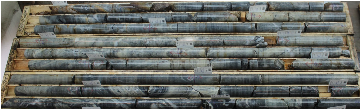
Photo 35: General view of the interval returning 4.22 ppm Au over 5 metres with minnesotaite occurrences and penetrative alteration
