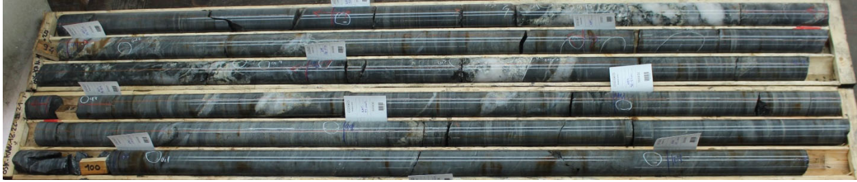
Photo 34: General view of veining in carbonate iron formation
