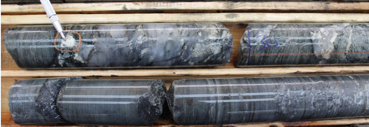
Photo 22: OSK-KAN-18-015 at 29.8 metres, Ankerite iron formation with 15% of quartz-ankerite-chlorite-pyrrhotite veins with several visible gold grains.
