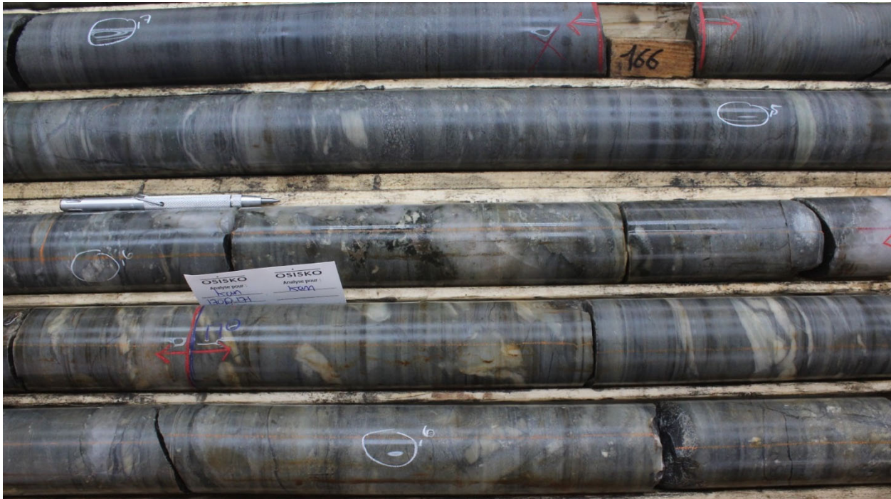
Photo 5: OSK-KAN-18-006 from 166 to 172 metres, Overview of carbonate iron formation, ankerite facies which returned a cut of 0.55 ppm Au over 17 metres.
