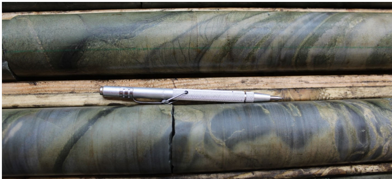
Photo 17: OSK-KAN-18-012 from 186.5 to 189.5 metres, Overview of the epidote alteration within the carbonate iron formation found in the hinge zone of the Ferricrete synform.
