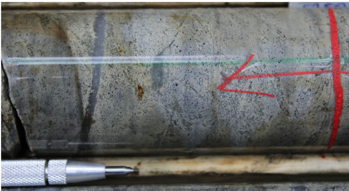
Photo 21: OSK-KAN-18-014 at 52.5 metres, Closeup of saccaroidal iron formation (possibly oxide chert?) with magnetite and pervasive pyrrhotite.
