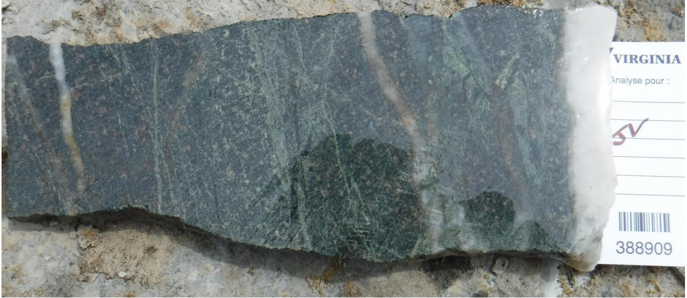
Figure 20: EJV2018TR008-G1 Altered granodiorite affected by chlorite-silica-epidote-hematite-magnetite alteration
