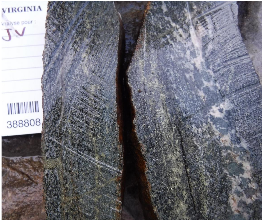
Figure 11: EJV2018TR004-G2 Diorite carrying 5% chalcopyrite, 1% malachite, 1% pyrite over 0.5 meter
