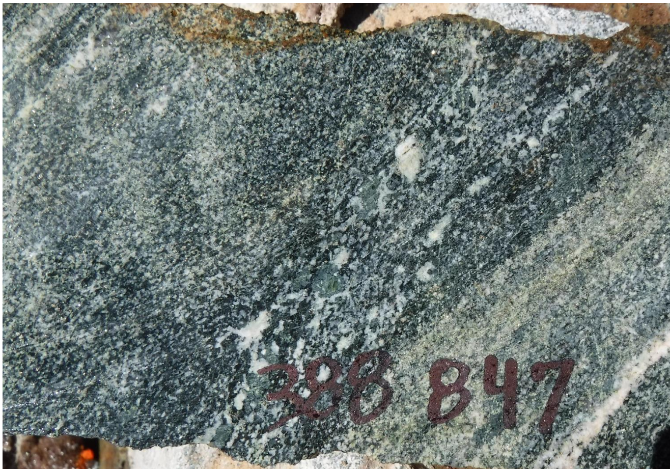
Figure 15: EJV2018TR006-G1 Diorite affected by moderate epidote alteration carrying 3-5% disseminated pyrite
