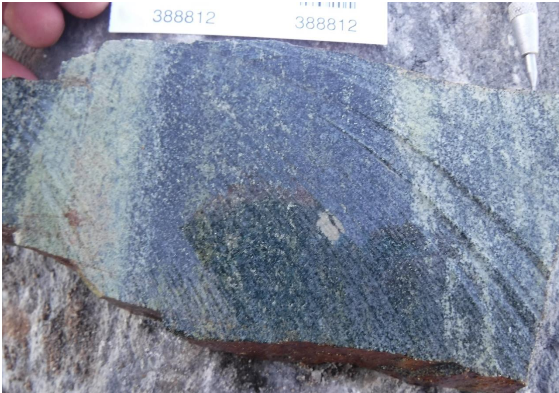
Figure 12: EJV2018TR004-R3 Diorite affected by epidote alteration and carrying 3-5% chalcopyrite, 3 % pyrite
