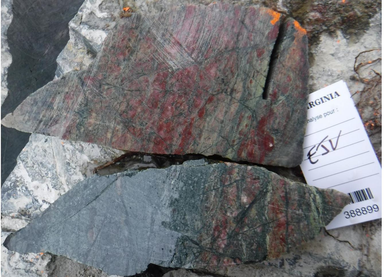
Figure 22: EJV2018TR008-R1 Chlorite-hematite-k-feldspar-epidote-silica altered granodiorite affected by multiple mm-sized crack-n-seal quartz veinlets
