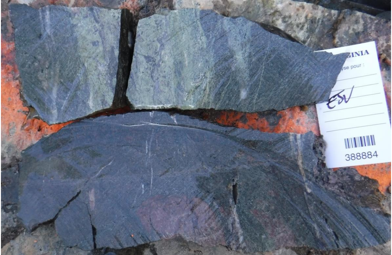
Figure 19: EJV2018TR007-R2; Altered granodiorite, epidote shear veinlets and a possible sub-rounded fragment
