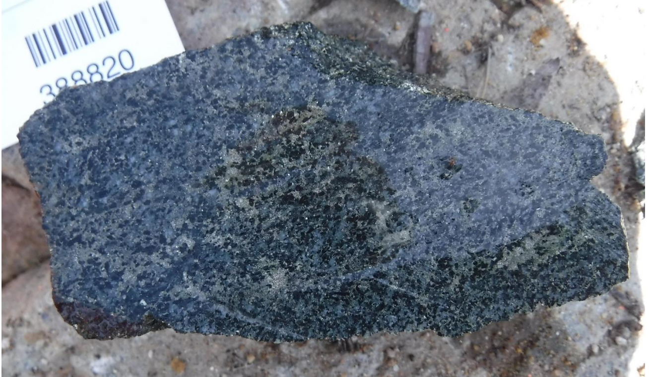
Figure 14: EJV2018TR005-R1 Medium grained diorite carrying 3-10% pyrite
