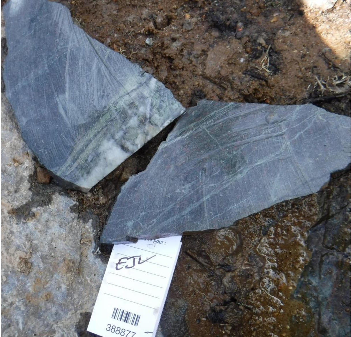
Figure 18: EJV2018TR007-R1: Highly altered in chlorite-hematite-magnetite granodiorite and an epidote veinlet brecciated by a quartz-hematite vein in the deformation zone.
