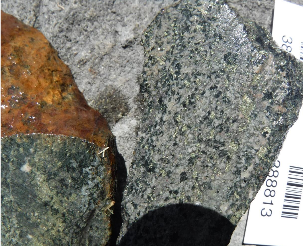
Figure 13: EJV2018TR004-R3 Medium grained diorite affected by epidote alteration and carrying 3-5% chalcopyrite, 3 % pyrite
